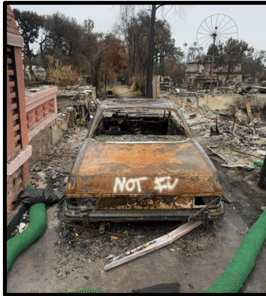
Figure J10. Burned car labelled “NOT EV” to designate it as a non-electric vehicle.
