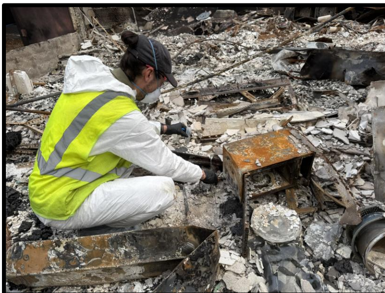
Figure J3. Sampling debris next to microwave as a “point source” sample.
