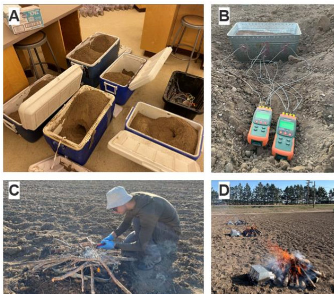
Figure 3.2. Pyrocosm assembly and ignition. (A) Mineral soil samples that were packed into the pyrocosms. (B) Pyrocosm being dug into a barren agricultural field with thermocouples inserted into the pyrocosm. (C) Igniting the pyrocosms. (D) Three replicates of burned pyrocosms.
