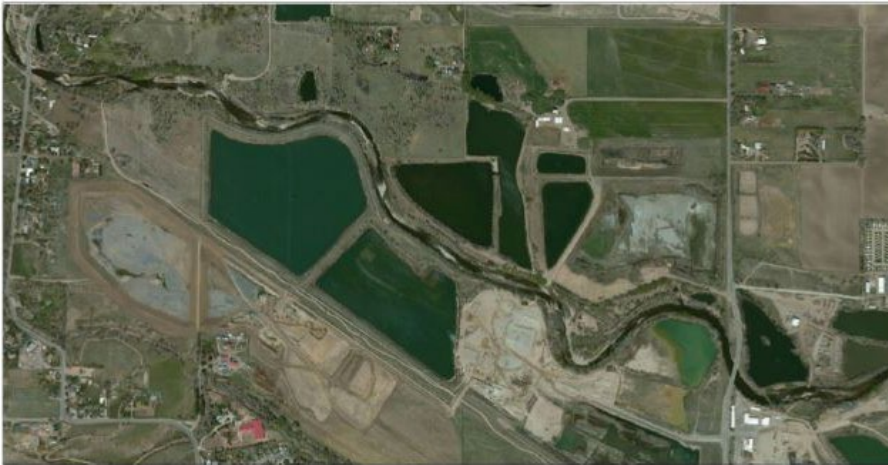
Figure 3. A 2.5 km long reach of the Poudre River in Fort Collins, CO, downstream of Lions Park (a) in 1937 and (b) 2005. (a) shows a multithread, laterally unconfined channel with an active and accessible floodplain, while (b) shows a confined, leveed, single thread channel with little lateral mobility, floodplain, or riparian forest. Flow is left to right in each image. From Bestgen et al. (2020) Figure 2
