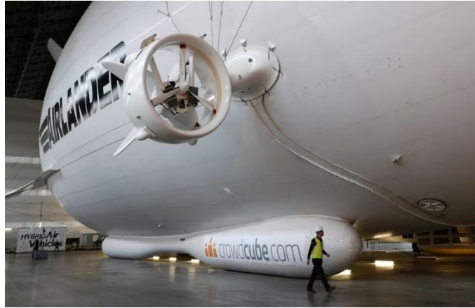
Figure 35: Airlander 10 Side-Mounted Propulsor [71]
