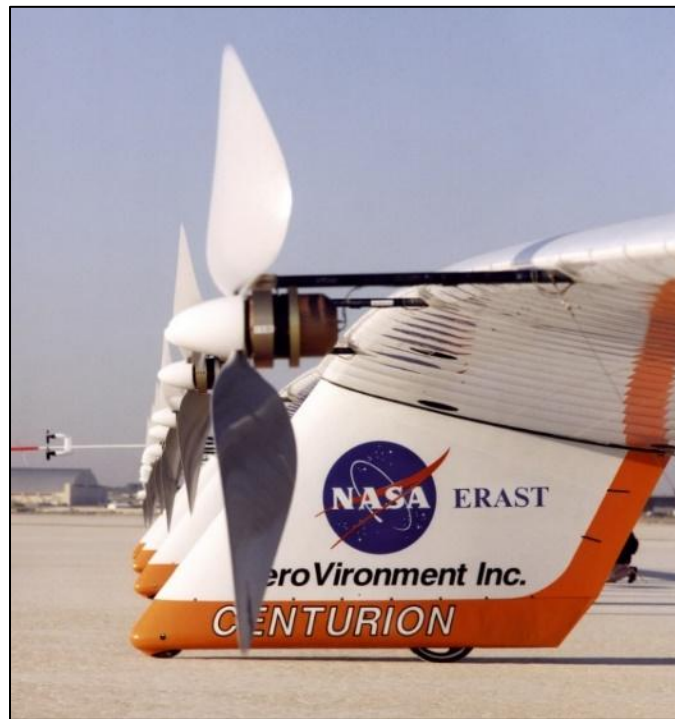
Figure 37: High-Twist Very High-Altitude Propellers [74]
