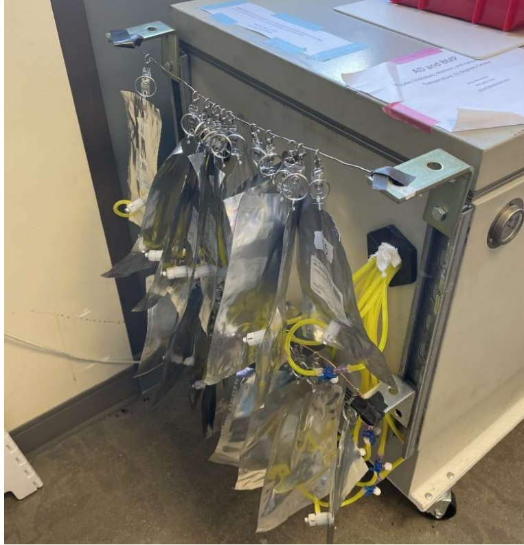
Figure 10: Gas collection bags located outside the orbital shaker.
