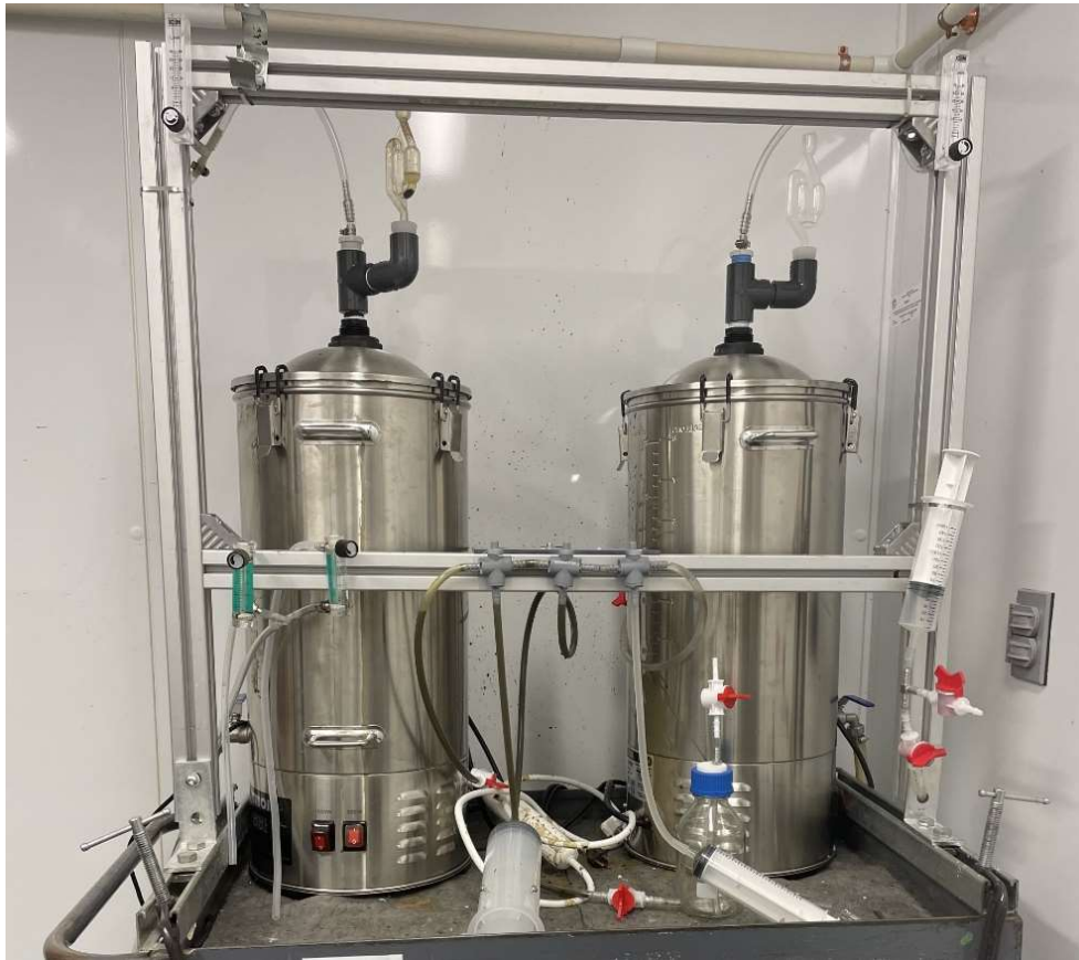
Figure 9: BMP Cart setup where BMP bottles were configured in an anaerobic system. The left container contained the inoculum and the right container contained nutrient medium.
