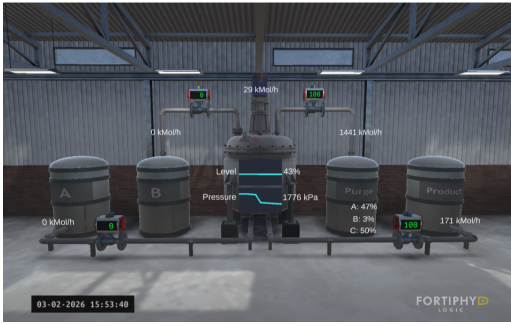
Figure 7: TE Process Plant’s Shutdown where Cyber-attack Triggers Pressure Sensor Failure (Fault) of Main Tank.
