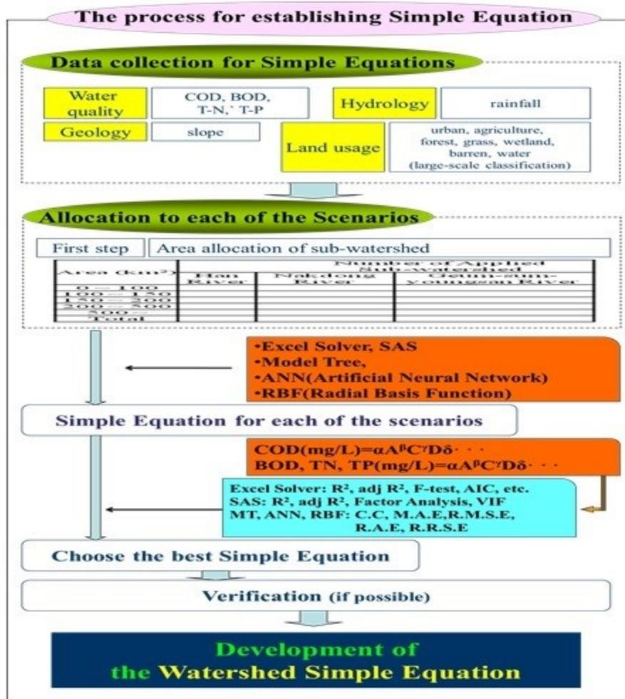
Figure 5-2: The process to establish Simple Equation to the new watersheds
