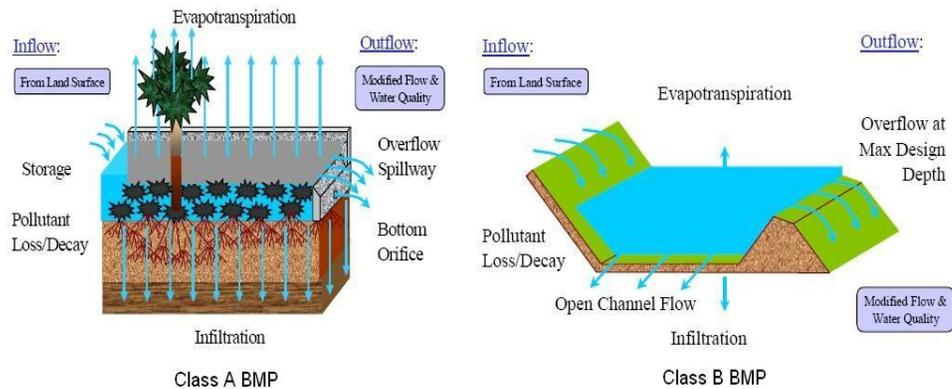
Figure A-9: BMP types of BMP Toolbox model (Cheng et al., 2004, 2009).
