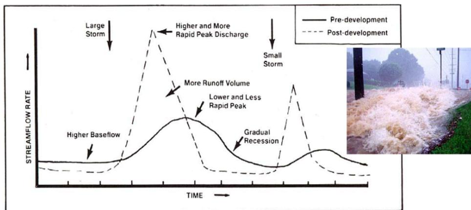
Figure 3-1: Comparison of pre and post development (Source: Schueler, 1987).
