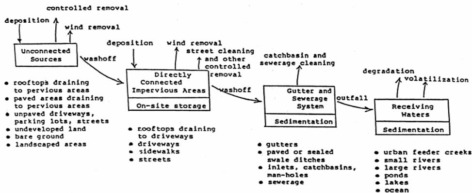
Figure A-11: The mechanism of pollutant deposition and removal at sources areas for SLAMM (Source: Pitt et al., 2000).
