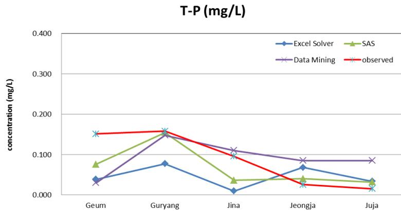
Figure 4-39: T-P simulation results based upon simple equations (Yongdam watershed).
