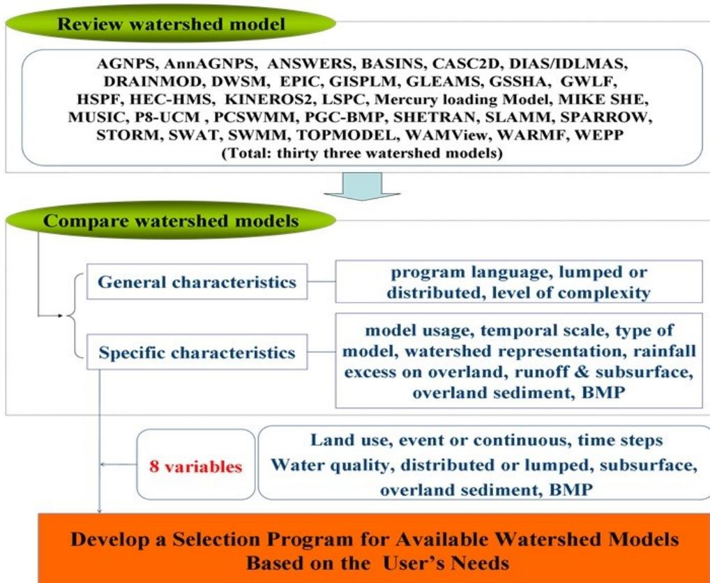
Figure 2-3: The Schematic for researching existing watershed models and developing a selection program.
