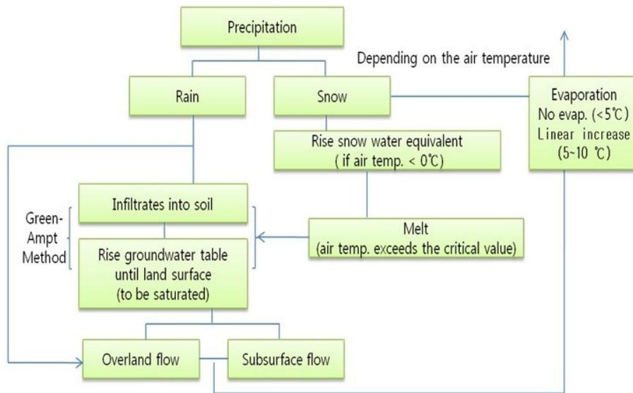
Figure A-17: Hydrological behavior of the catchment in TOPMODEL (Source: Holko et al, 1997).
