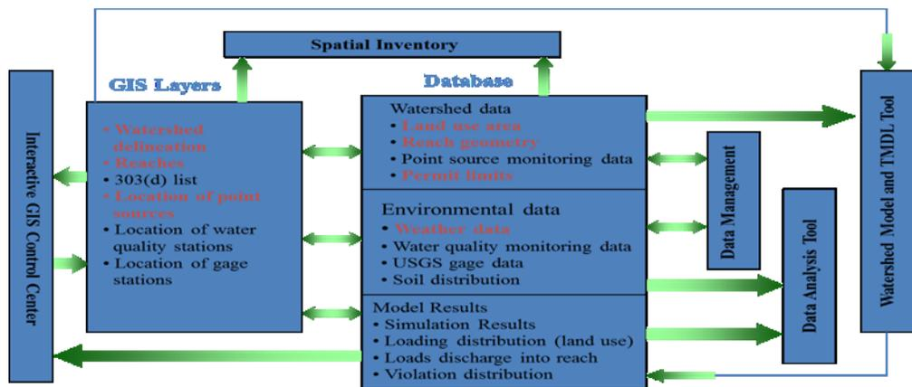
Figure A-4: LSPC (Loading Simulation Program in C++) Data Flow Schematic (Source: John Riverson).
