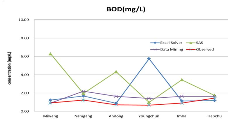
Figure 4-40: BOD simulation results based on simple equations (Nakdong watershed).
