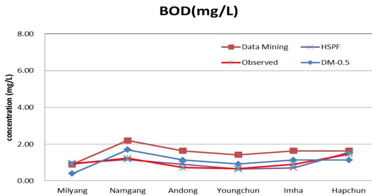
Figure 4-46: The results of BOD simulation for Nakdong river watershed based upon HSPF and simple equation.
