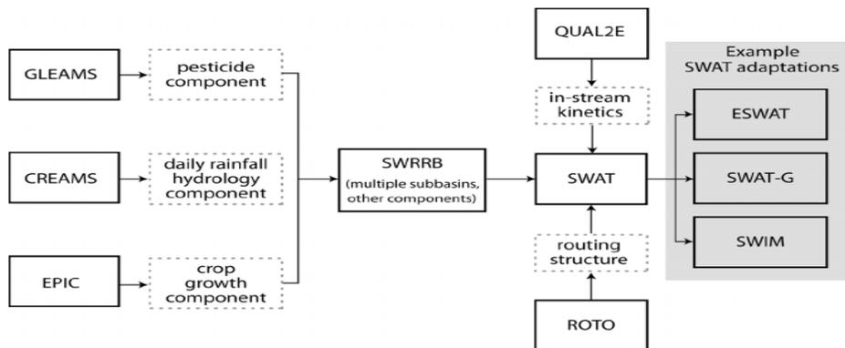
Figure A-14: The Schematic of SWAT's development (Source: Gassman et al, 2007).
