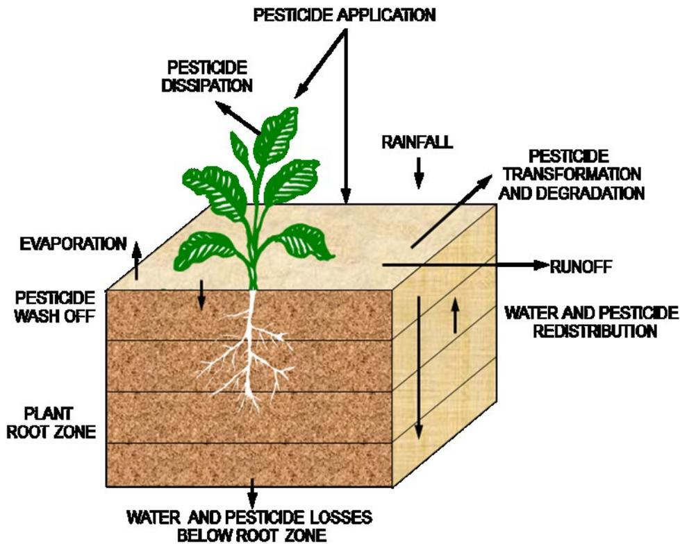
Figure A-3: The physical system and processes represented in GLEAMS.
