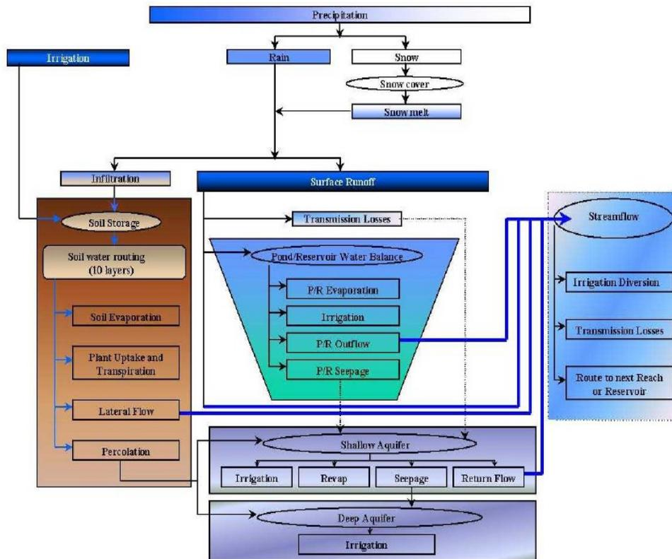
Figure A-15: The Schematic of a potential water pathway of the SWAT model (Neitsch et al., 2005).
