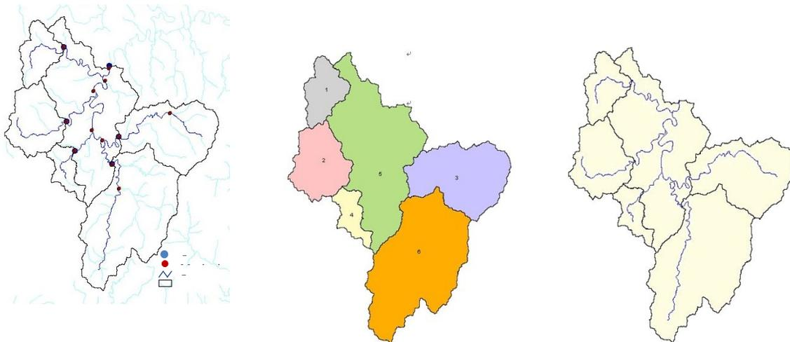
Figure 4-15: Outlet location, watershed delineation, and generated stream network at Yongdam Dam Watershed.
