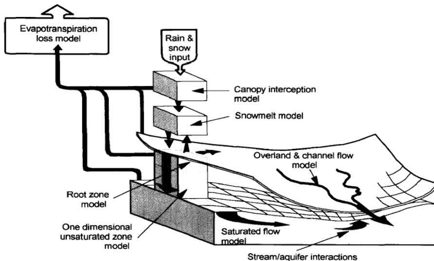
Figure A-10: Flow schematic diagram of SHETRAN model (Source: Dunn et al., 1996).
