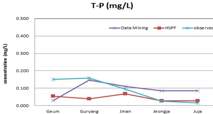
Figure 4-45: The results of T-P simulation for Yongdam Dam watershed based upon HSPF and simple equation.
