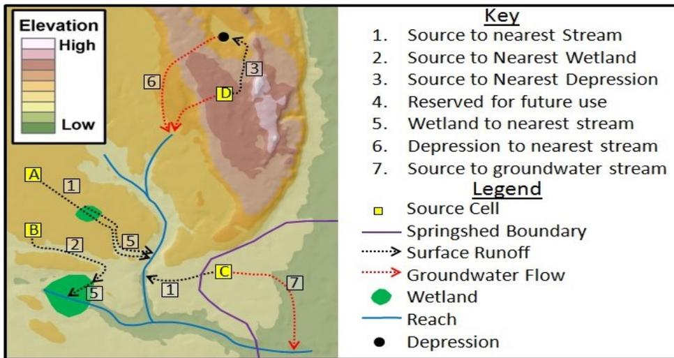
Figure A-18: The distance grid creation of flow and load generation.
