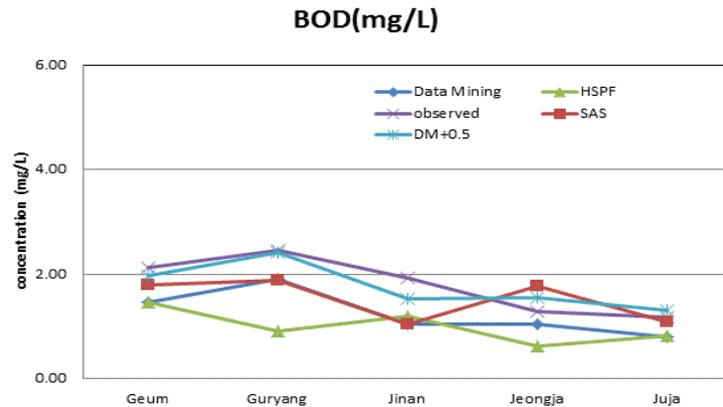
Figure 4-43: The results of BOD simulation for Yongdam Dam watershed based upon HSPF and simple equation.
