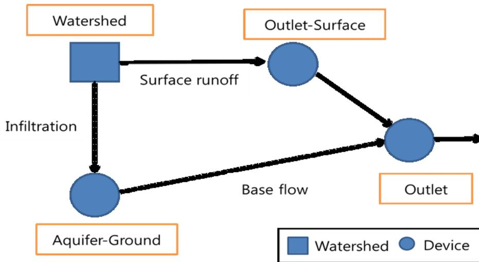
Figure A-8: Simple P8-UCM set up (Source: Tetra Tech, Inc., 2005).
