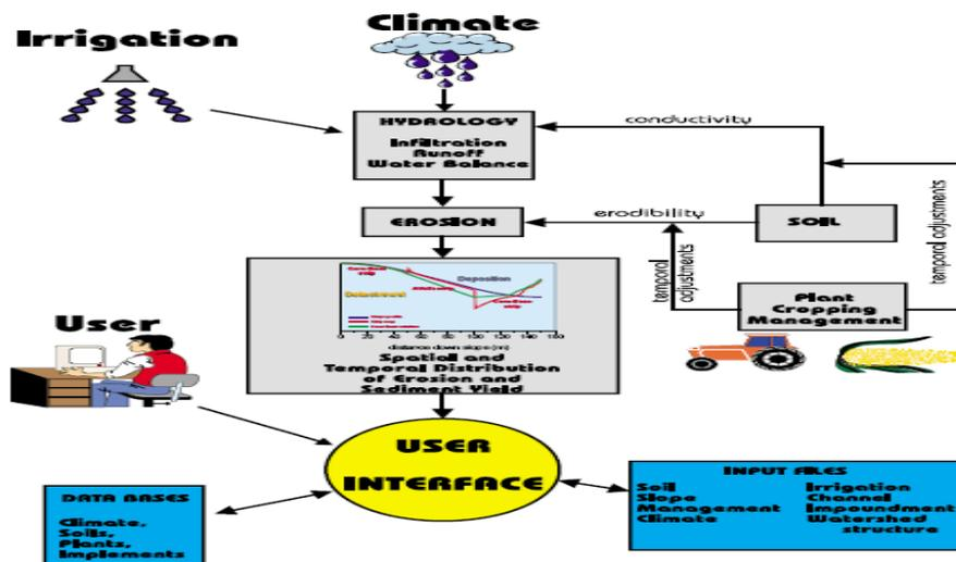
Figure A-21: The process schematic of the WEPP model (Source: Flanagan et al., 1995).
