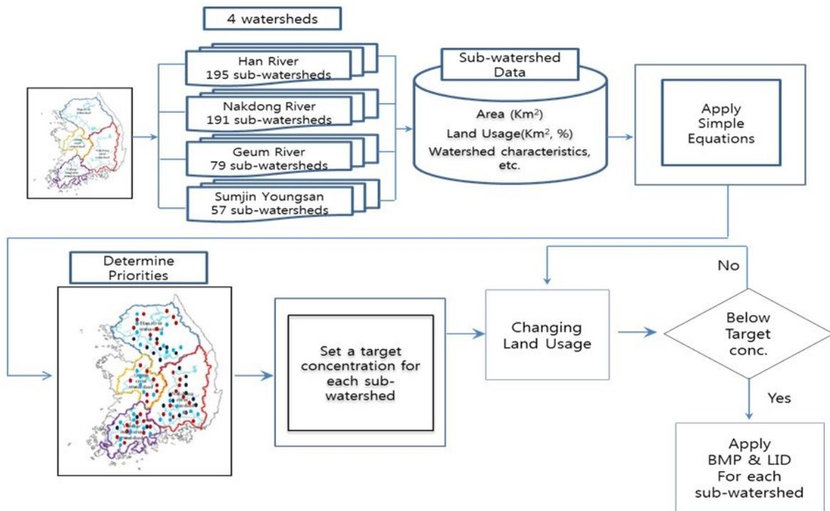
Figure 5-1: Future research schematic for sub-watershed management based upon Simple Equations.
