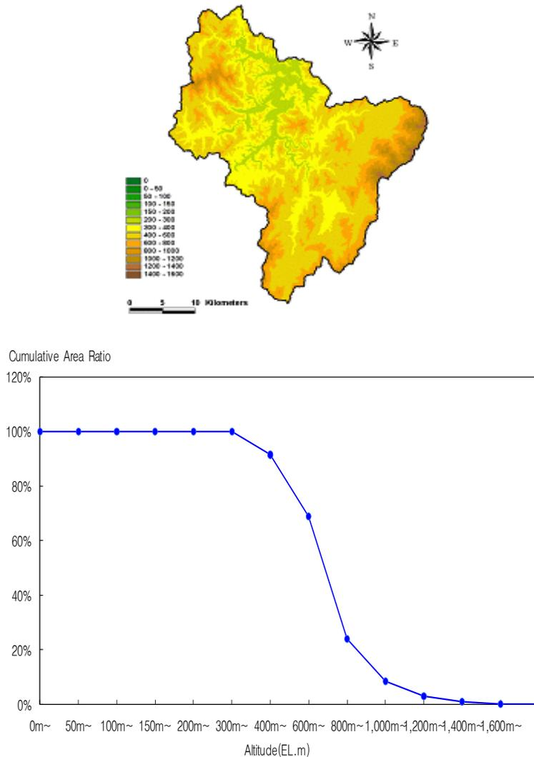
Figure C- 1: The altitude analysis map and the accumulative area ratio for the altitude analysis
