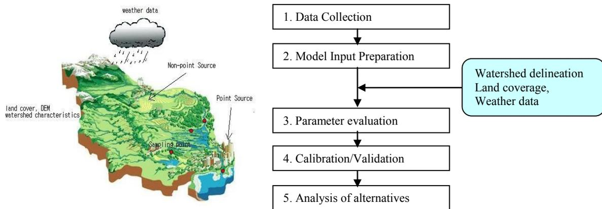
Figure 2- 1: The process of application for watershed model.
