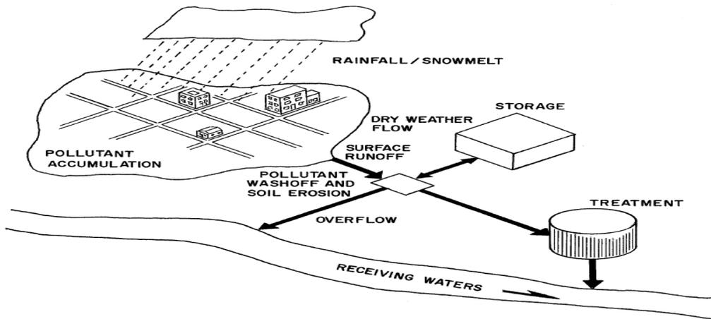
Figure A-13: The schematics of STORM model's flow mechanism (U.S. ACE, 1997).
