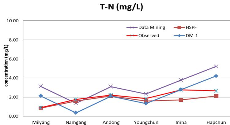
Figure 4-47: The results of T-N simulation for Nakdong river watershed based upon HSPF and simple equation.
