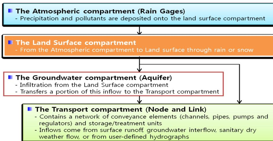
Figure A-16: The SWMM model’s Schematic (Source: Rossman, 2010).
