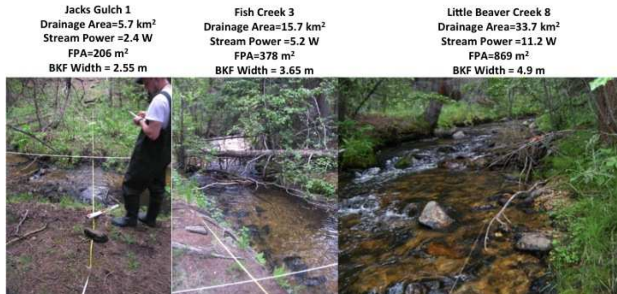
Figure 5.21: Principle component 2 spectrum in photographs. Along PC2 drainage area increases, stream power increases, floodplain area increases, and bankfull width increases. PC2 is roughly the size and slope of the drainage area.
