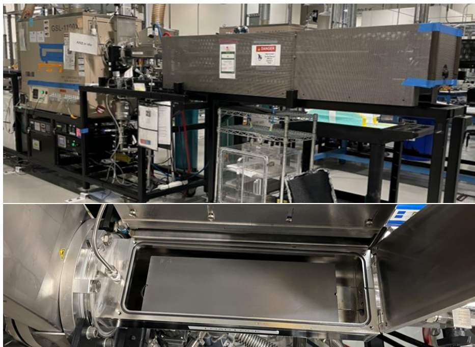
Figure 2.4: Furnace used in CHT and group-V activation steps showing the magnetic transfer arm, load lock, and processing chamber. Interior of load lock showing graphite crucible sitting on end effector of the MTA.
