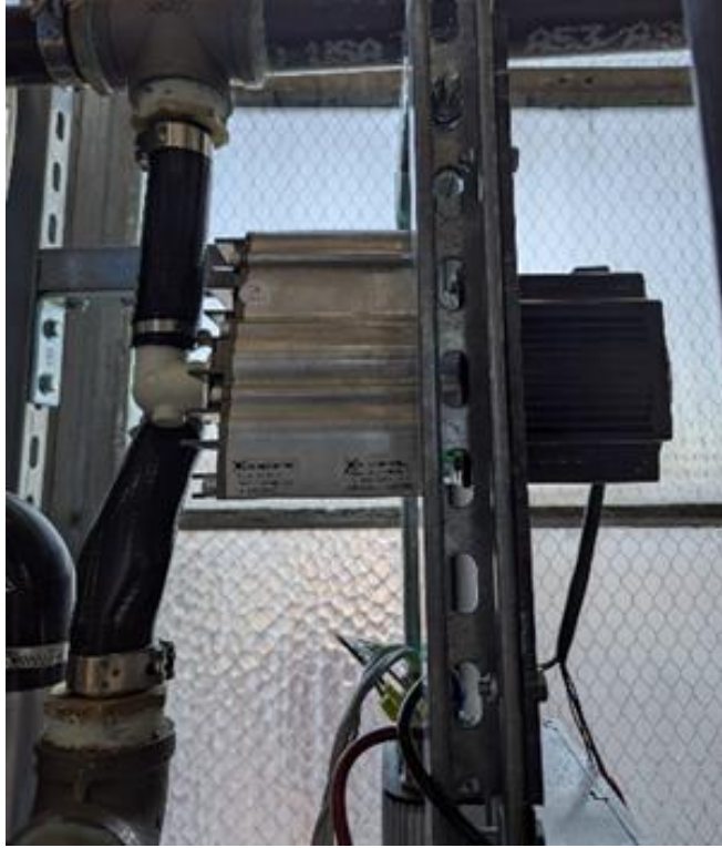
Figure 10. Air Squared P24H056A-BLDC supercharger.
