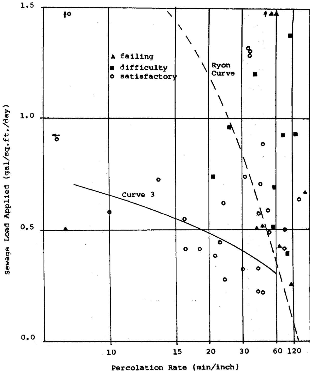
FIGURE 12 FIELD LOADING SUCCESS AS A FUNCTION OF PERCOLATION RATE
