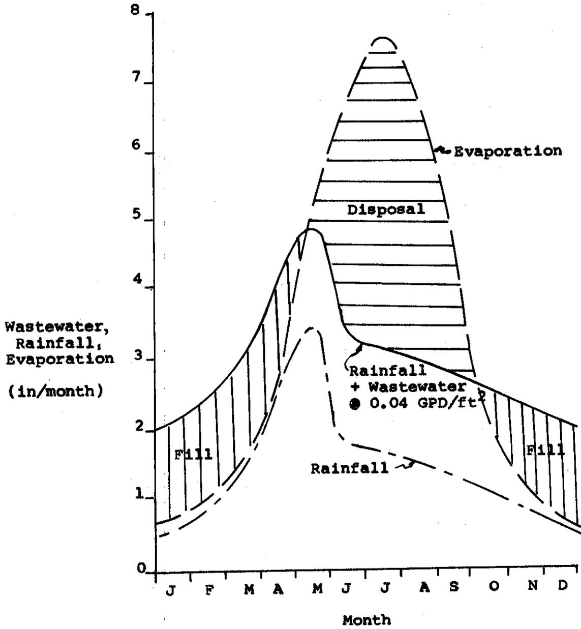
FIGURE 21 TYPICAL E-T POTENTIAL CURVE
