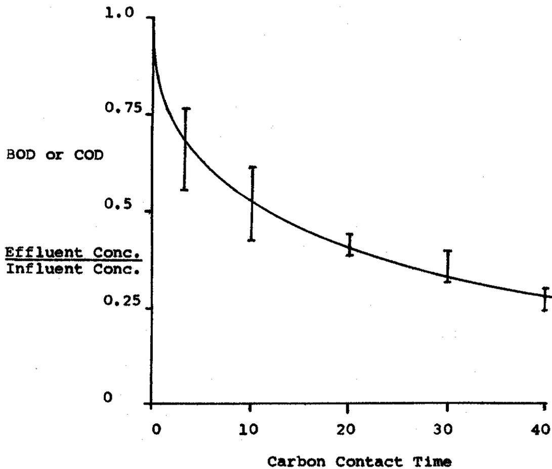
FIGURE 26 BOD AND COD REMOVAL WITH ACTIVATED CARBON
