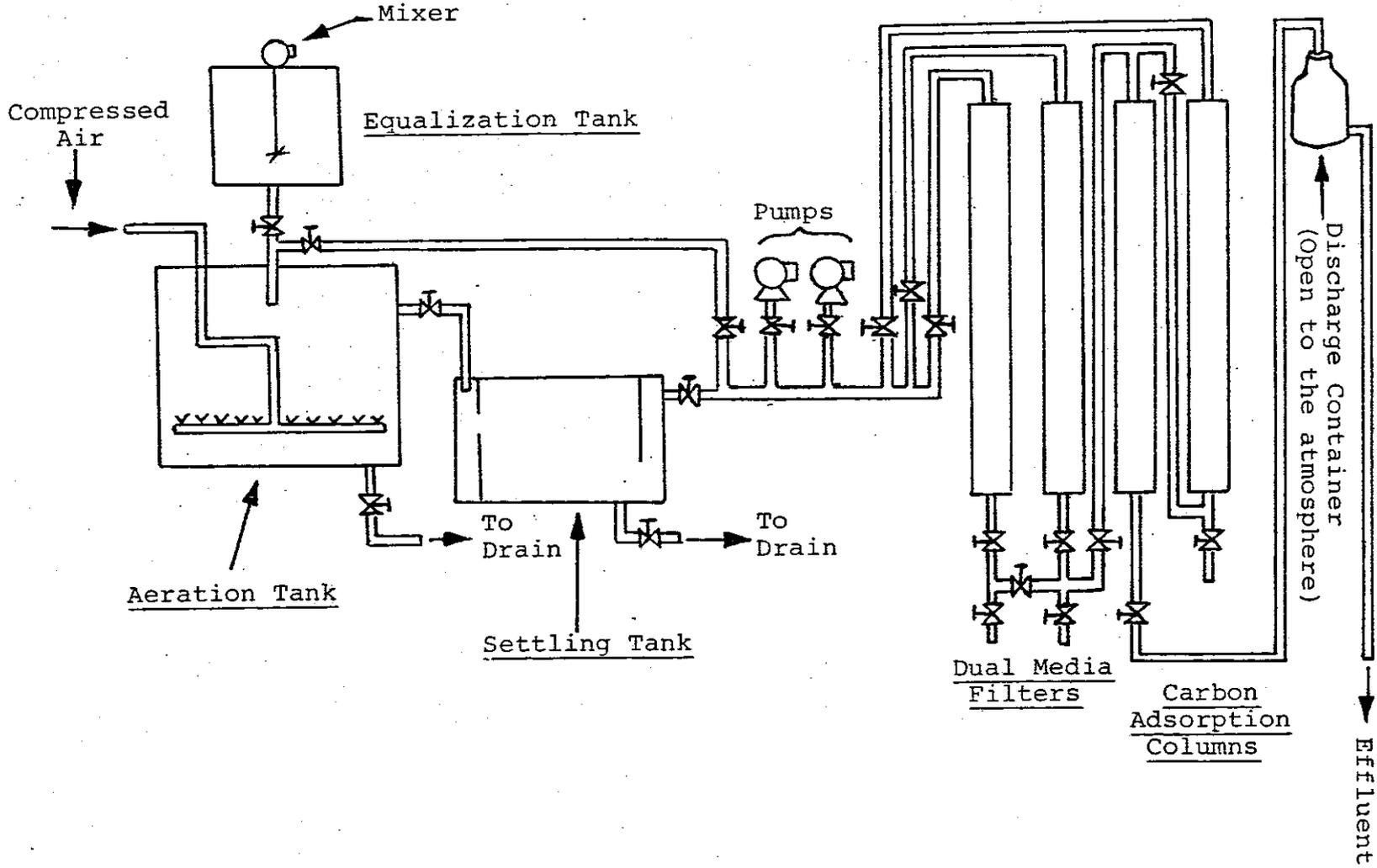
FIGURE 25 DIAGRAM OF BENCH SCALE PILOT PLANT
