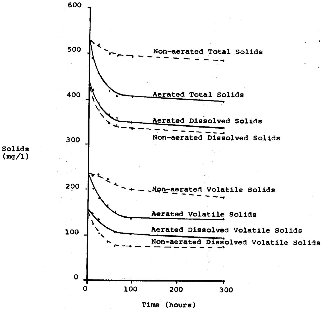
FIGURE 23 COMBINATION WASTES SOLIDS REMOVAL CURVES
