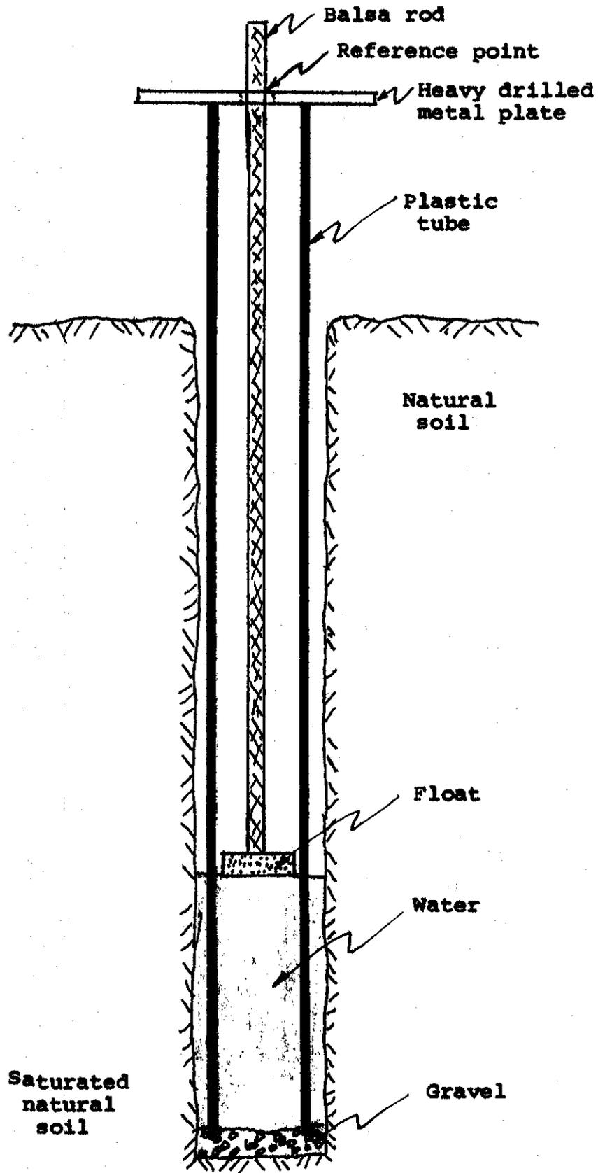
FIGURE 13 DEVICE USED FOR PERCOLATION TESTS
