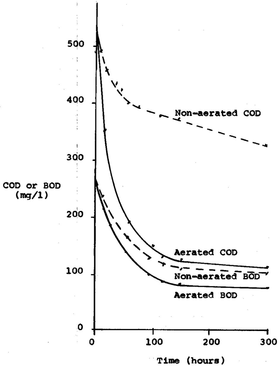
FIGURE 24 COMBINATION WASTES COD,BOD REMOVAL CURVES
