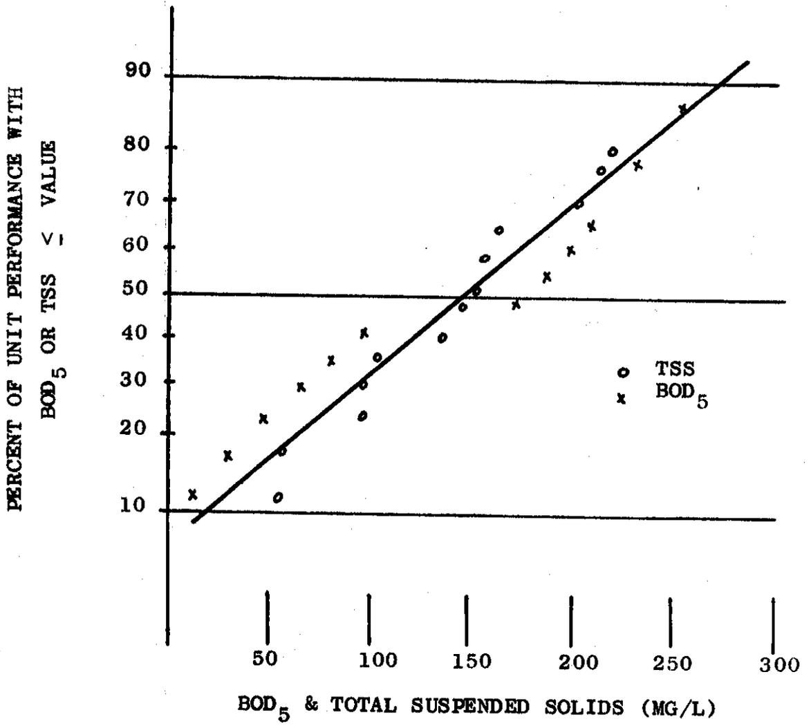
FIGURE 18 SPOT CHECK EFFLUENT QUALITY OF SEVERAL FIELD UNITS
