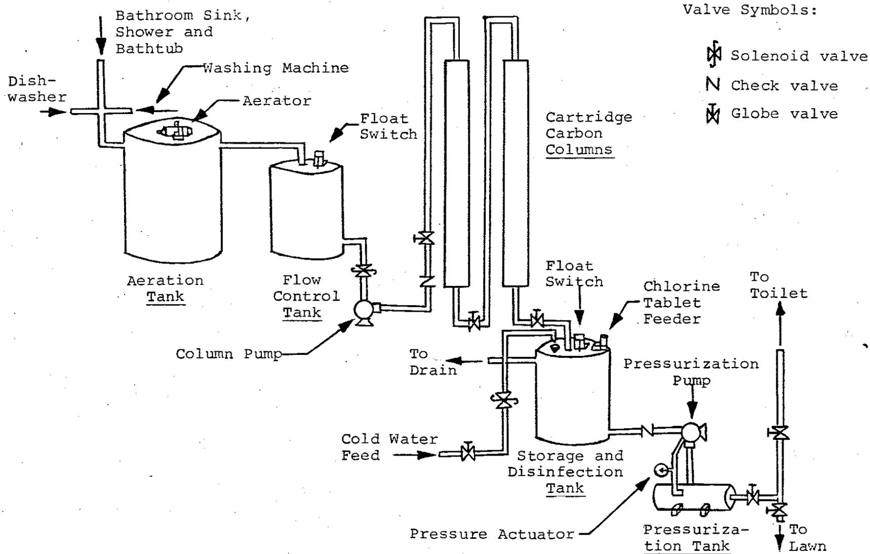
FIGURE 27 AERATION-CARBON ADSORPTION TREATMENT SYSTEM
