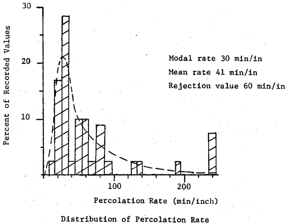
FIGURE 15 PERCOLATION TEST VARIATIONS IN DECOMPOSED SHALE
