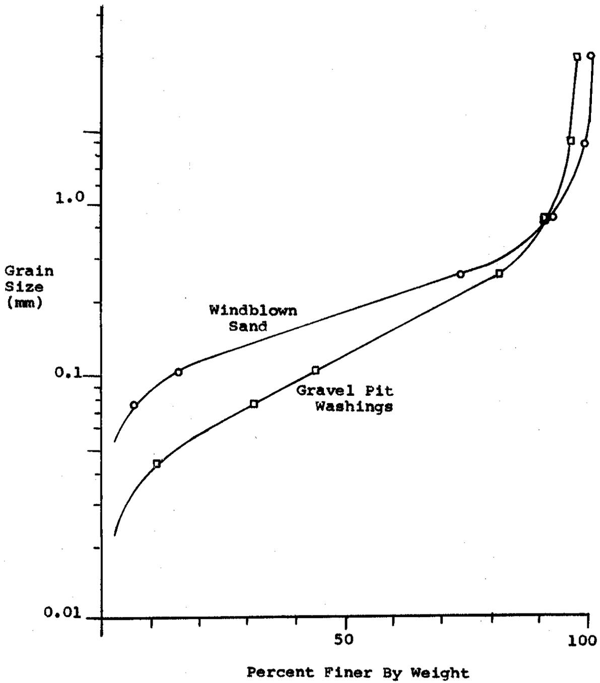
FIGURE 20 E-T SOIL SAND SIZE SIEVE ANALYSIS
