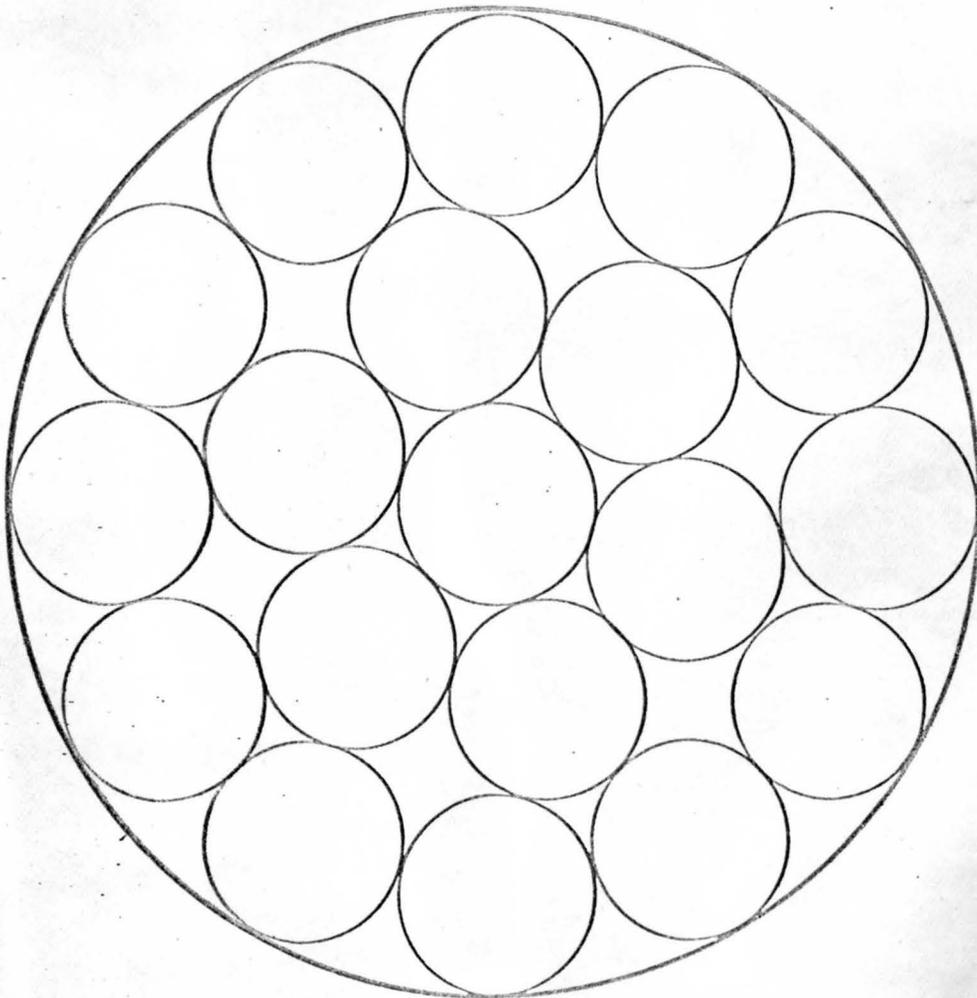
Cross-section of flow straighteners for 26" pipe
