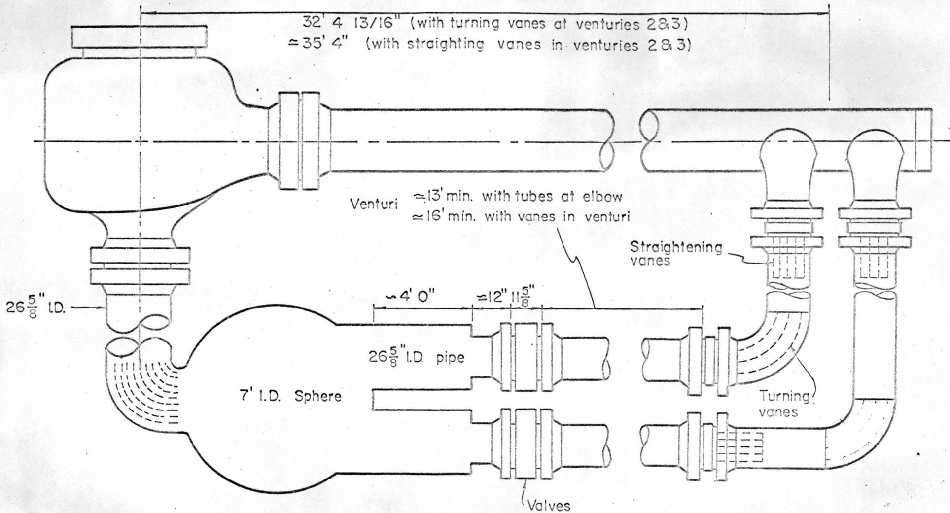
Figure 2. Schematic of proposed permanent modifications.
