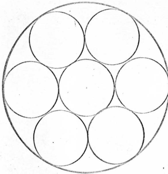
Cross-section of flow straighteners for 16" pipe
