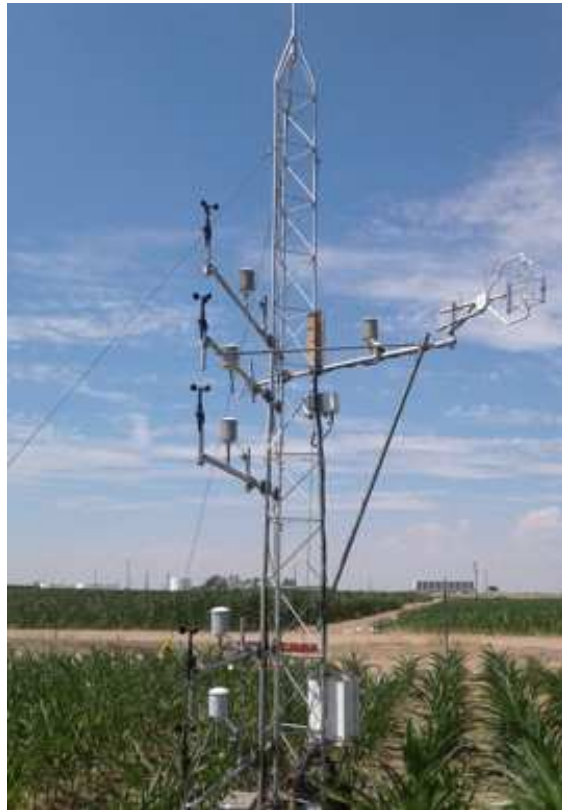
Figure 3.20: The EC system at LIRF in 2017 (Field E) with aerodynamic profile sensors (e.g., cup anemometers and hygrometers).
