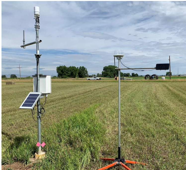
Figure 3.15: The ClimaVUE50 IIC weather station in a non-pristine grass. Photo provided by Ansley Brown.
