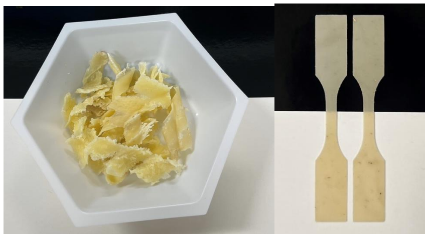
Figure D61. Digital images of LDPE-PLLA (50/50 wt%) + UDC3 (5wt%) blend extrudate flakes (left) and dogbone tensile specimens generated from reprocessing post-tensile test specimens (right). The original blend of LDPE-PLLA (50/50 wt%) + UDC3 (5wt%) was first compounded via melt-extrusion, and the blend extrudate was reprocessed via compression molding into dogbone specimens for initial tensile tests. After these tensile tests, the broken pieces were mixed with 50wt% virgin LDPE and melt-extruded, and the resulting blend extrudate (now 75/25 wt% LDPE-PLLA + 2.5wt% UDC3) was once again compression-molded to the reprocessed/recycled dogbone specimens (right image) for additional tensile tests. The results were reported in Figure S65.
