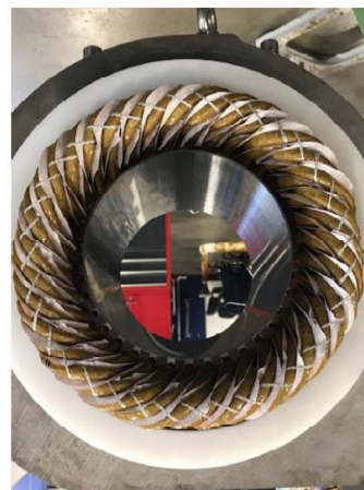
(b) Stator assembly
