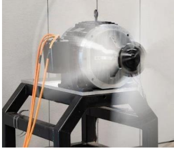
Figure 42 Hinetics Subscale Demo for 5 MW Motor
