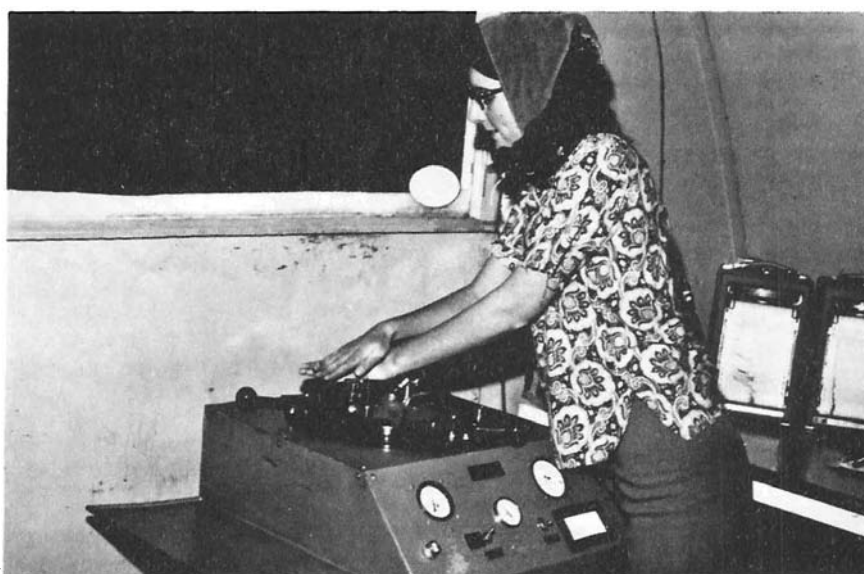
Fig. 4 Operation of Bigg-Warner Ice-Nuclei Counter
