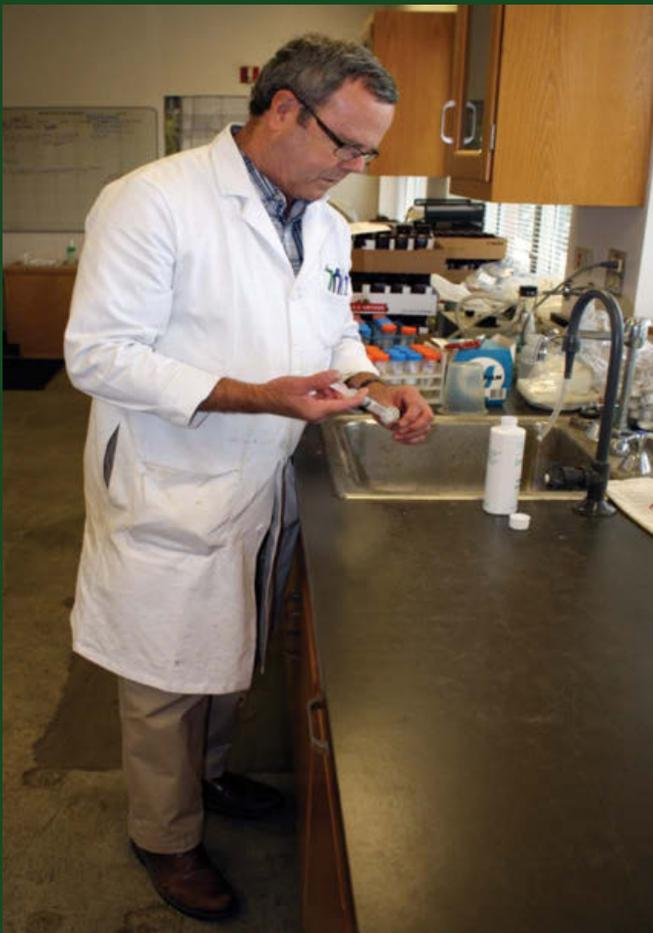
*Jim Self filtering a water sample in the CSU water lab to prepare it for analysis. Samples are usually filtered prior to analysis unless the testing requires a non-filtered sample.*
