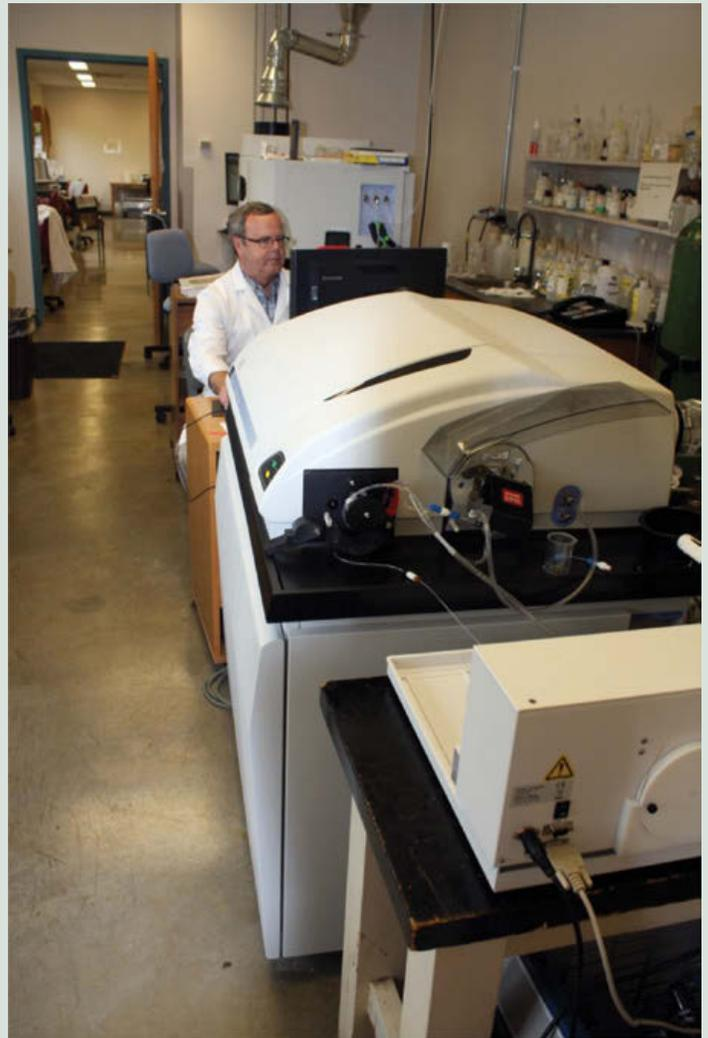
*Jim Self operating the inductively coupled plasma-mass spectrometer (ICPMS) in the CSU water lab. The ICPMS is capable of measuring elements at the part per billion or part per trillion level.*
