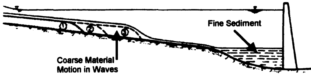
Figure 2-5. Motion of Coarse Material Waves illustrated by 1, 2, and 3 along the Longitudinal Profile (From Simons and Sentürk, 1992)
