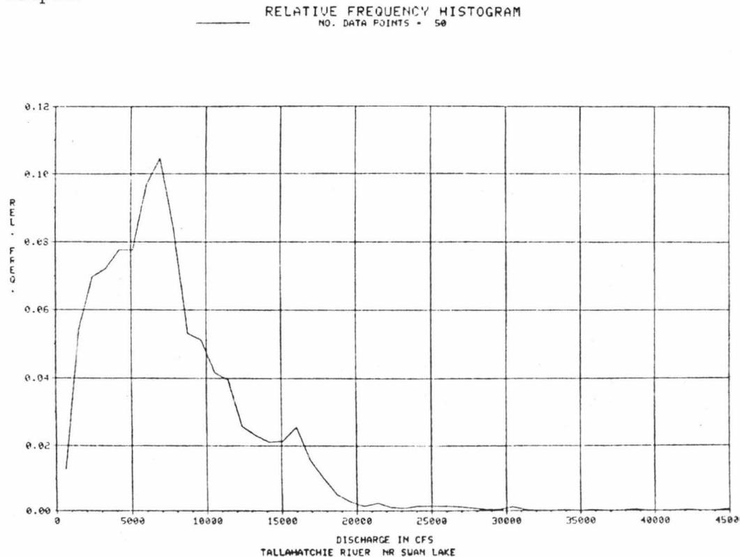
EXAMPLE 40: All discharge data for a frequency analysis (both cumulative and relative) for a gaging station.
