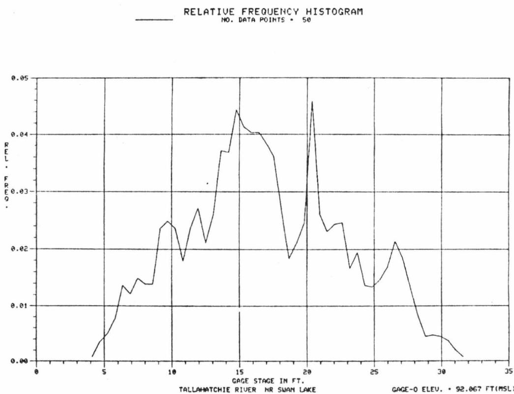
EXAMPLE 24: River stage data for a frequency analysis (both cumulative and relative) for a gaging station.
