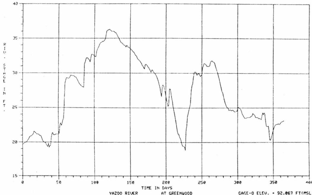
RETRIEVAL AND PROCESSING OF DISCHARGE-HYDROGRAPH DATA
