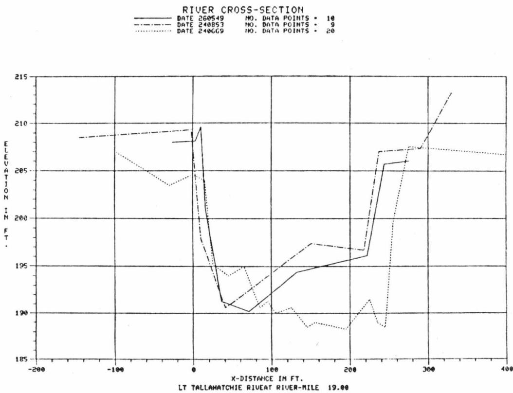
EXAMPLE 58: Cross-section plot for a gaging station for a specified date.
