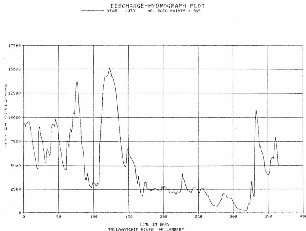
EXAMPLE 32: Discharge plot for a gaging station for a specified time.
