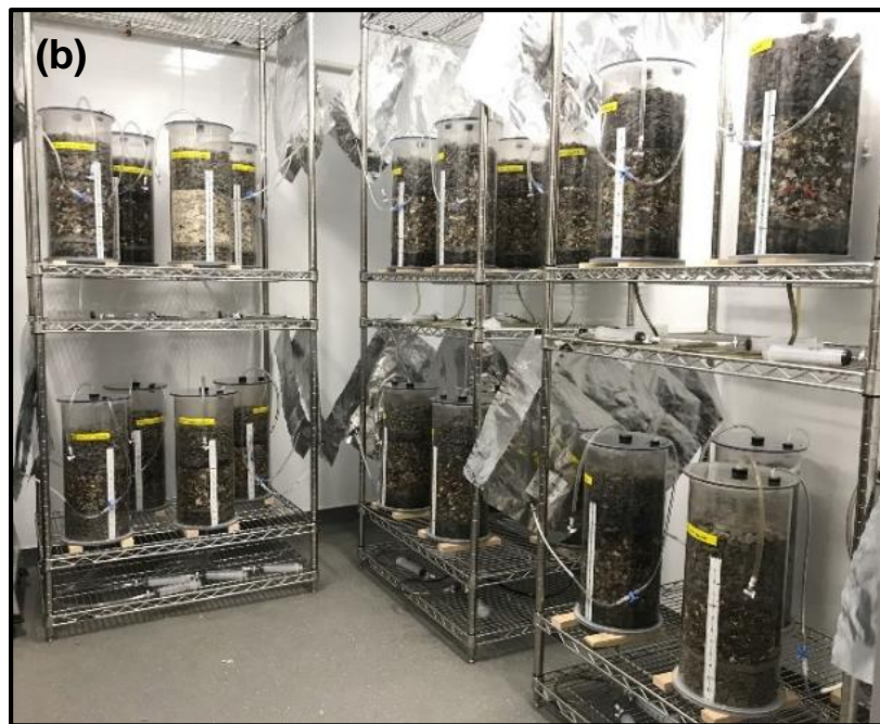
Figure D-2. (a) Final constructed control reactors and (b) temperature control room with 24 reactor experiments in operation.
