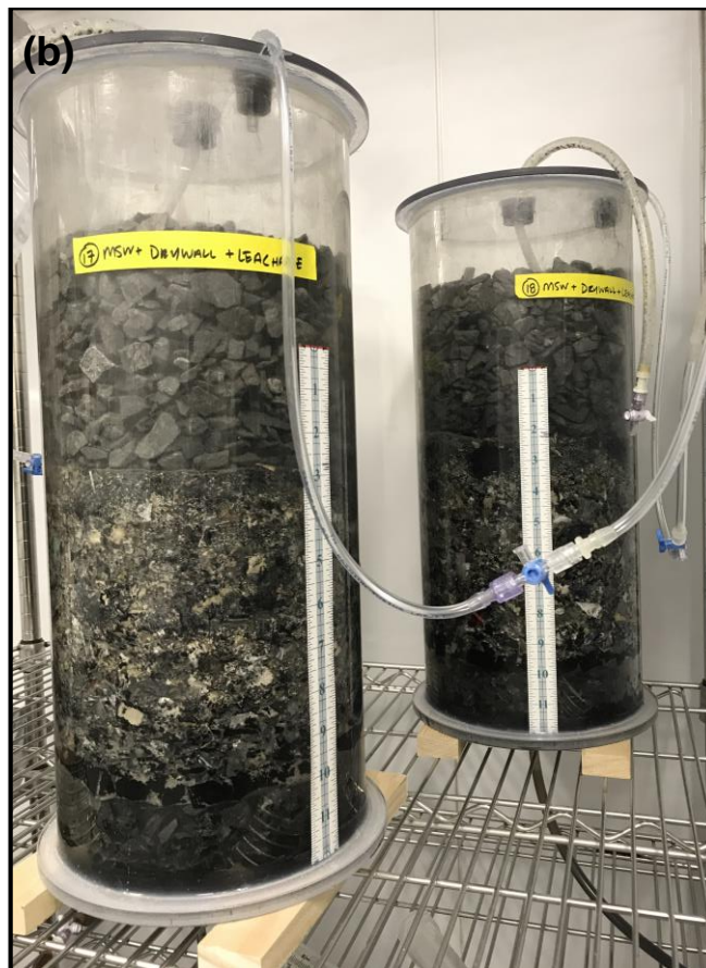
Figure D-6. Operational considerations including (a) reactor clogging due to AD sludge addition and (b) sulfate reduction, indicated by the black coloration in the GB reactors.
