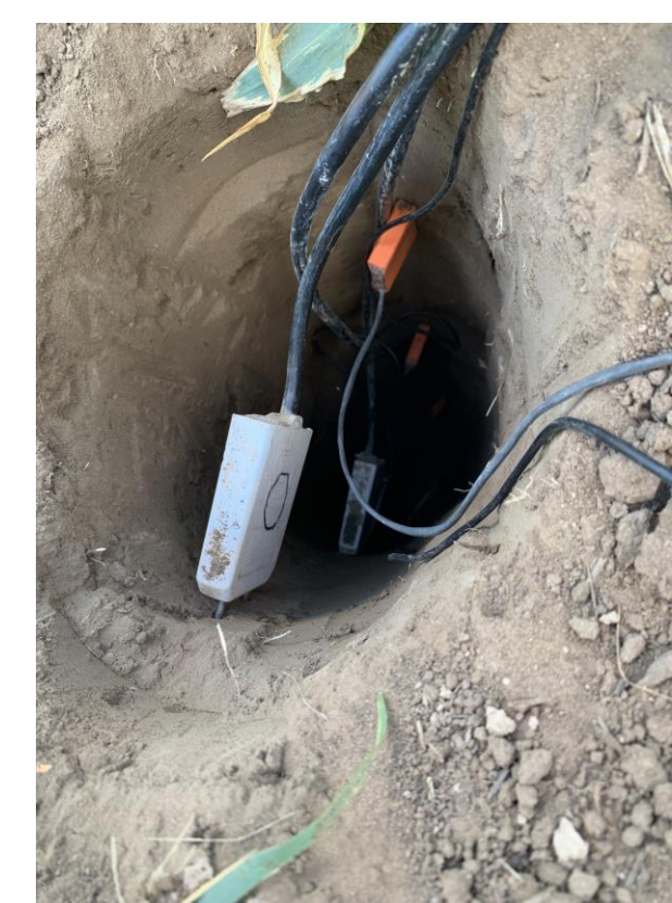
Commercial and DIY sensor stuck into soil profile
