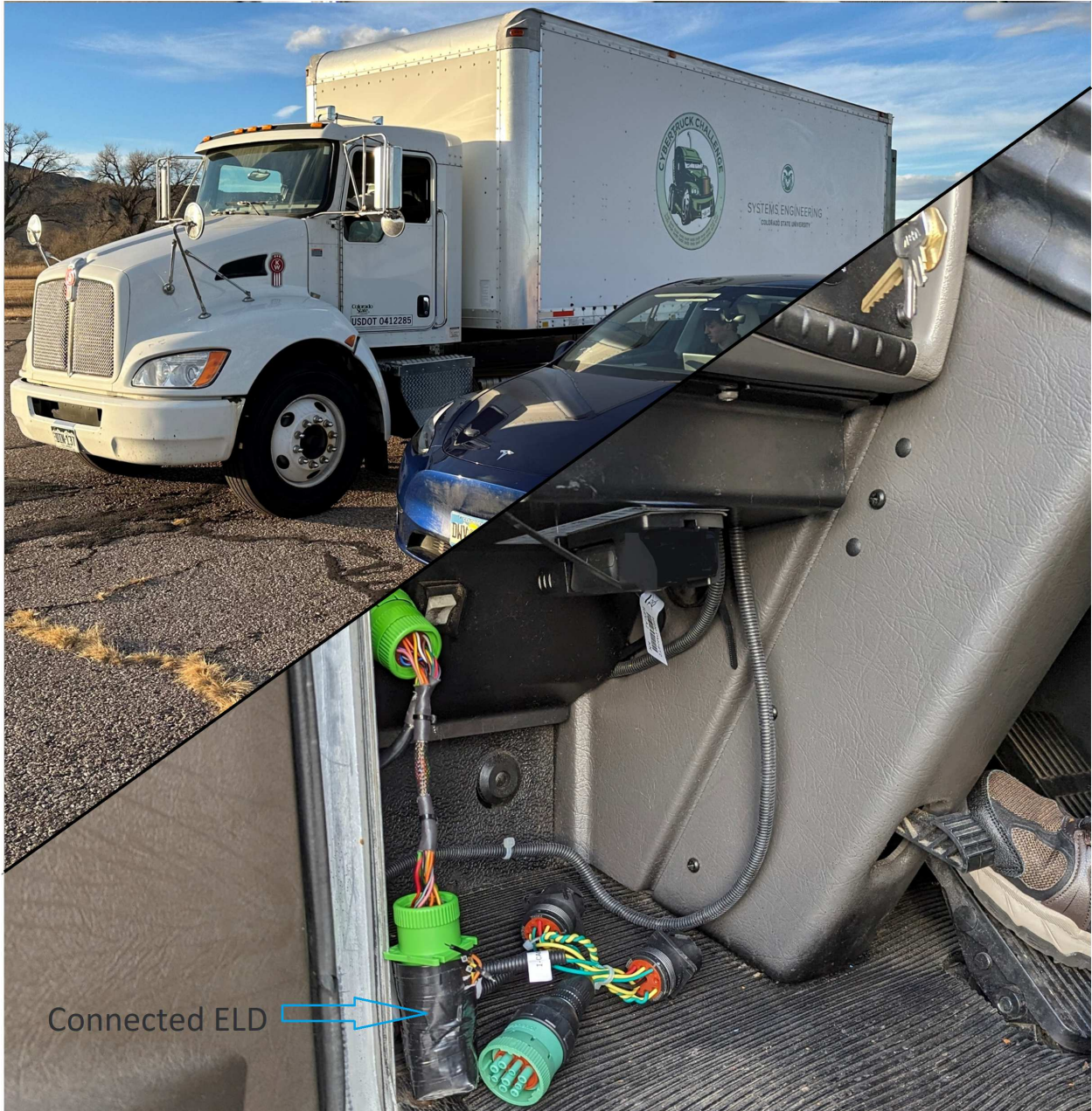
Figure 2.10: Research Truck (top) with ELD plugged into Diagnostic Port and hanging to the right of the door edge (bottom).
