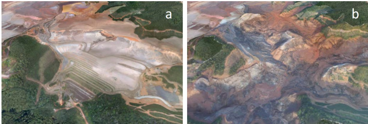
Figure 3.6 – Fundão Dam before (a) and after failure (b) (Morgenstern et al., 2016)
