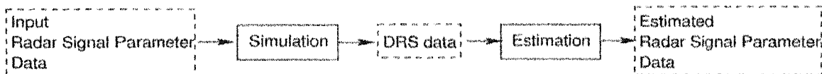
Figure 4.3: Procedure to confirm the DRS simulation and the radar signal estimation algorithms.
