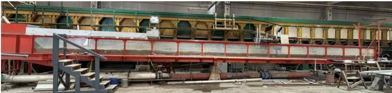
Figure 2. 18.3 m x 0.6 m x 0.6 m recirculating laboratory flume at Colorado State University Hydraulics Lab.
