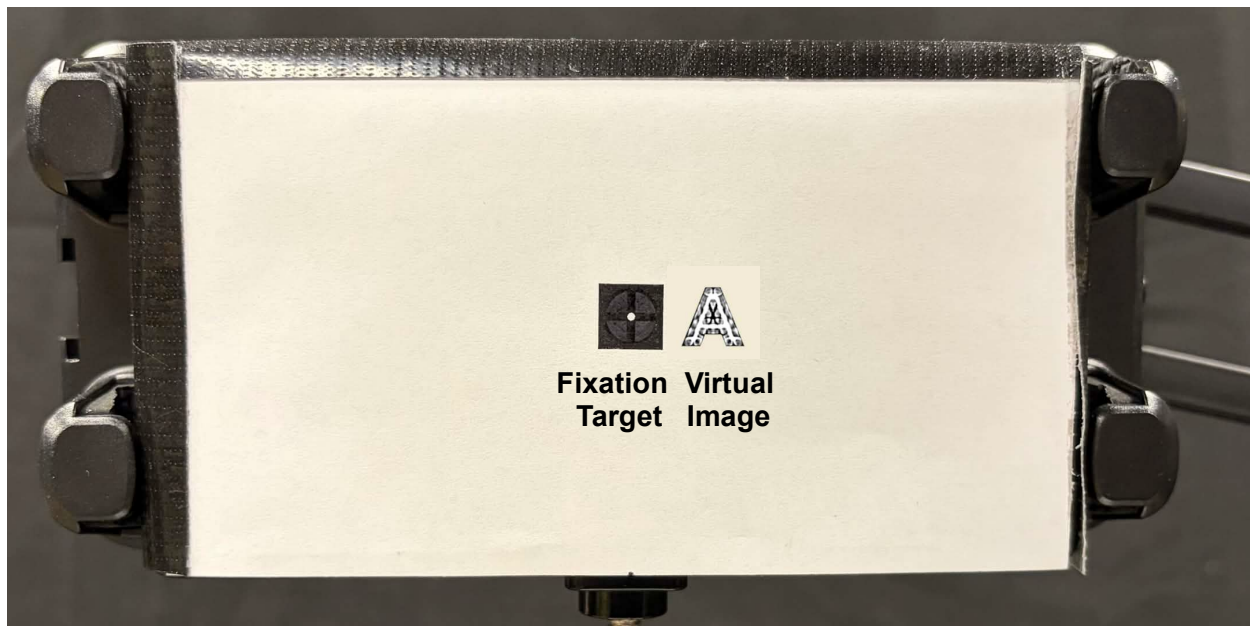
Figure 4.3: Stimuli presented to participants, consisting of a fixation target (left) and a SharpView-processed virtual image (right).
