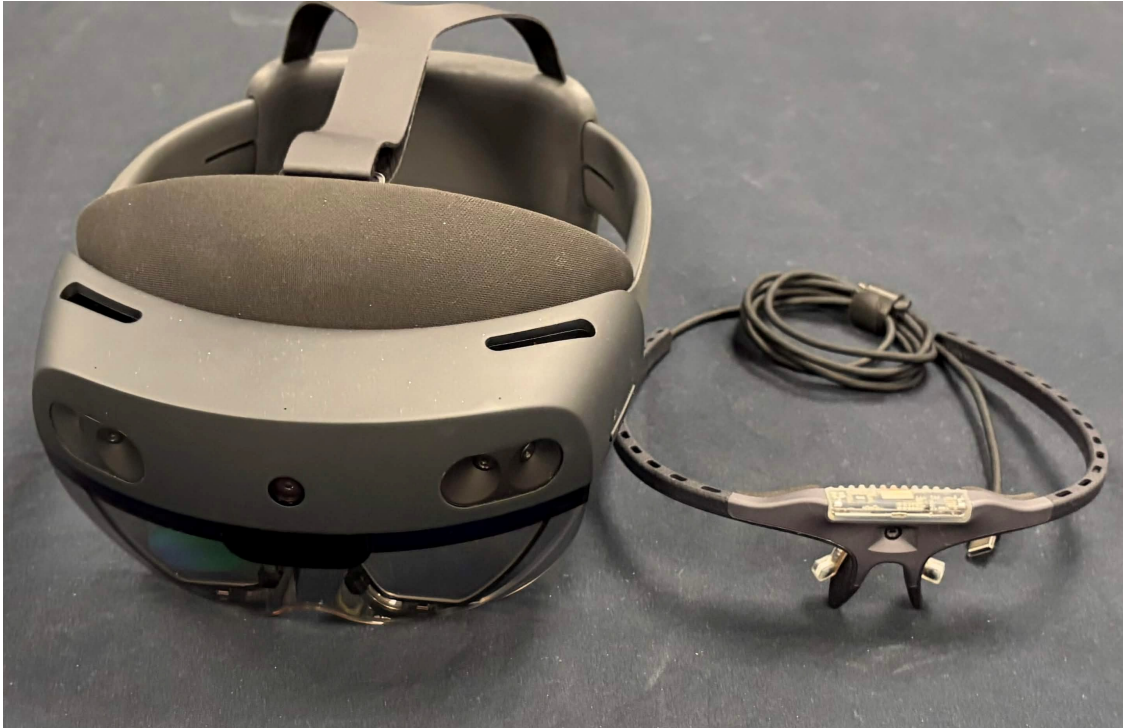
Figure 4.4: Apparatus used in this study: Microsoft HoloLens 2 (left) and Pupil Labs Neon (right).
