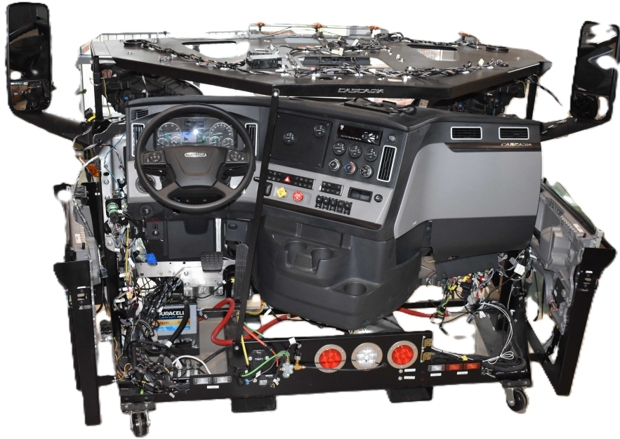
Figure 4.5: Freightliner Cascadia Cab Testbed
