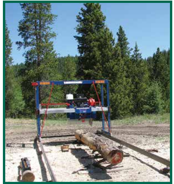
A portable sawmill is just one tool that can be used to create higher-value wood products.
