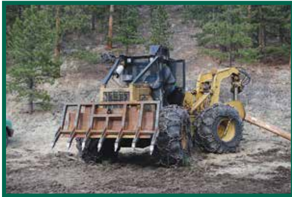
A skidder with a brush rake on the front is an efficient way to build slash piles.
