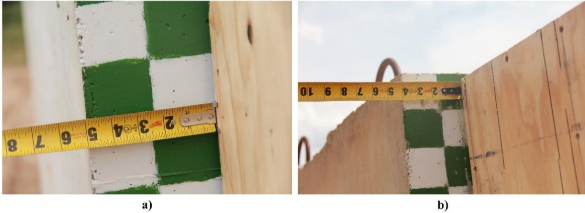
Figure 6-13: a) Checkerboard gauge pretest measurement and b) barrier permanent deflection of 0.024m (1in) from experiment 5 posttest.
