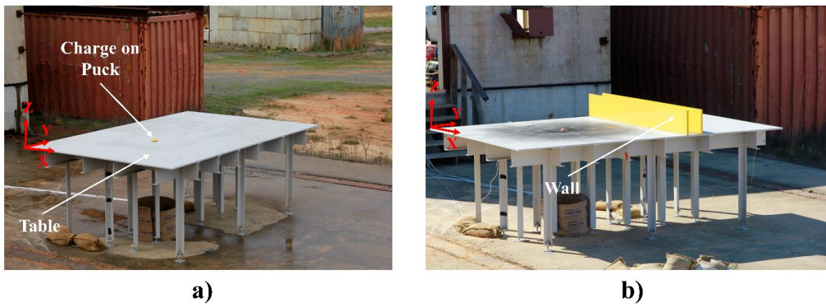
Figure 3-2: Steel rectangular table used for small-scale testing of a) free fields and b) multi-wall experiments.
