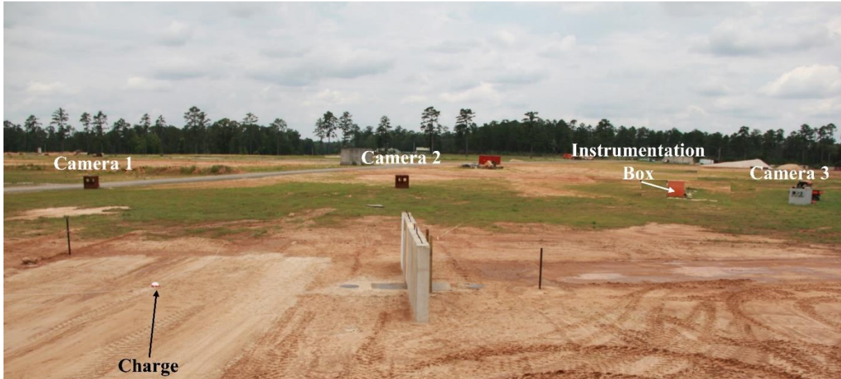
Figure 6-8: Field location of all three high speed cameras relative to the barrier structure.
