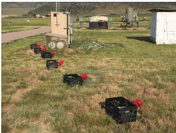
(a) Six Sierra flow meters connected in series at the CSU Methane Testing and Evaluation Center. (b) Pressure regulators and Omega flowmeter used for Sierra meter verification
