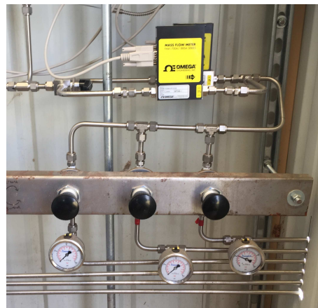
(a) Six Sierra flow meters connected in series at the CSU Methane Testing and Evaluation Center. (b) Pressure regulators and Omega flowmeter used for Sierra meter verification
