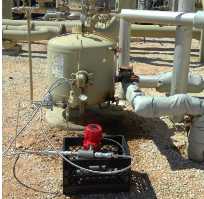
Figure 4.1: Emission measurement system installed on supply gas line to PC controlling liquid level in a secondary liquids storage tank.
