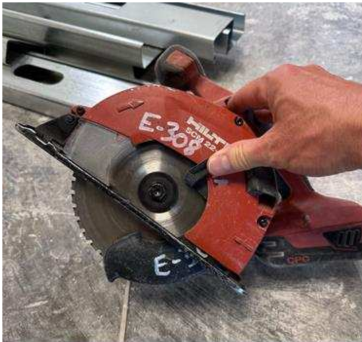
Fig. 1.5. Detail of the metal-cutting blade on the cordless circular saw.
