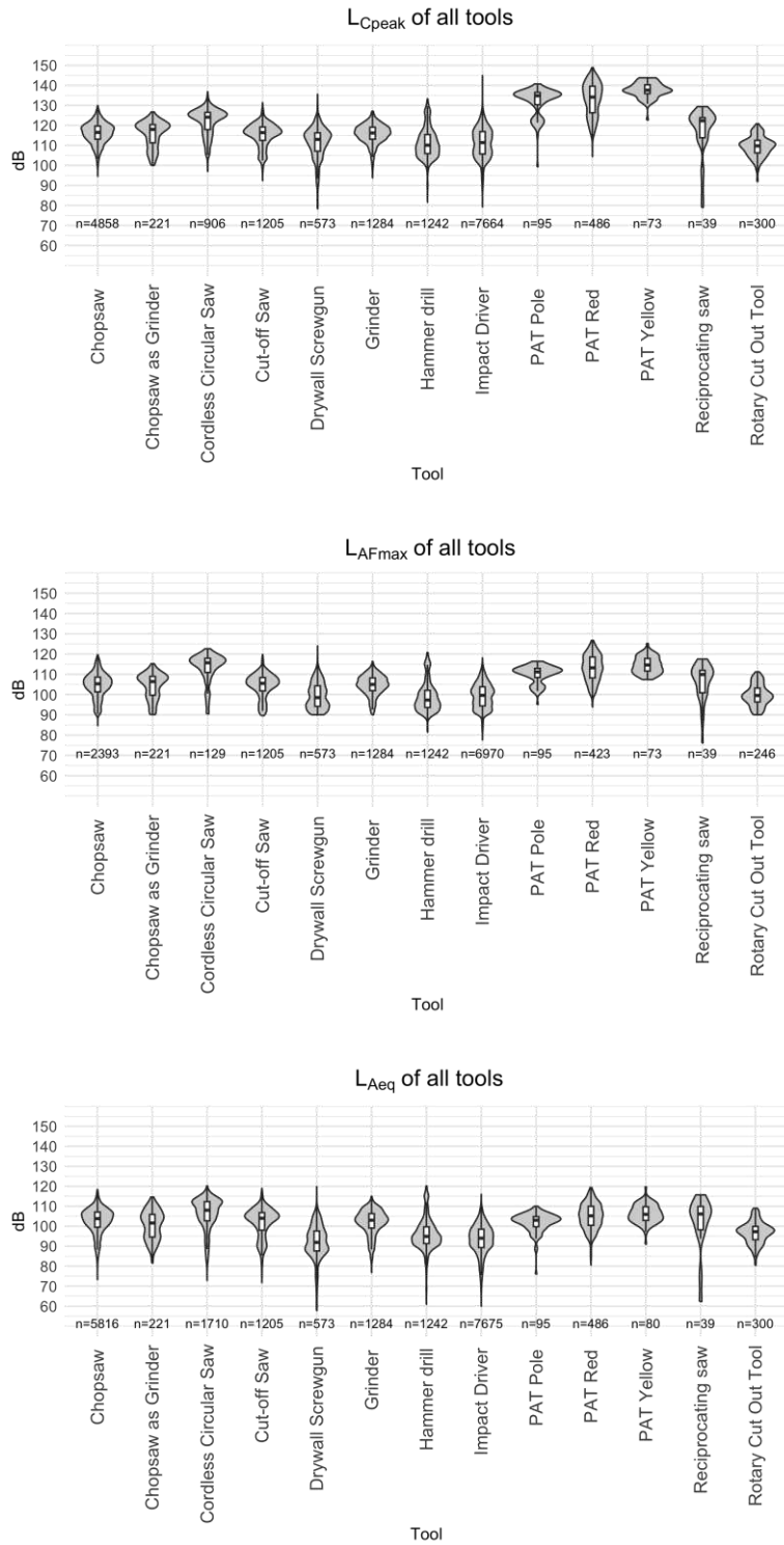
Fig. 2.5. Noise metrics for each tool used by the workers in the study. Sample size indicates number of 1-second samples the dosimeter recorded for each tool. For boxplots: Horizontal line = median, boxes = interquartile range (IQR), whiskers = 1.5*IQR.
