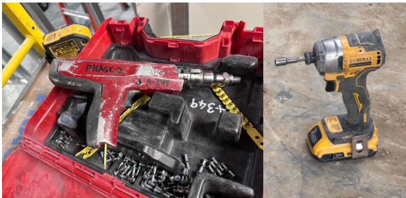
Fig. 3.2. Typical common tools used by framers in the study. Powder-actuated tool (PAT) nailer (left) and impact driver (right).
