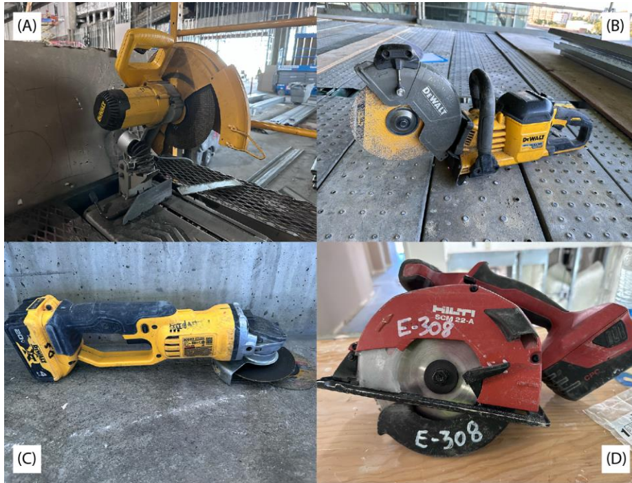
Fig. 1.2. Examples of each saw type that was used at the study sites. A = Chopsaw; B = Cut-off Saw; C = Grinder; D = Cordless Circular Saw.
