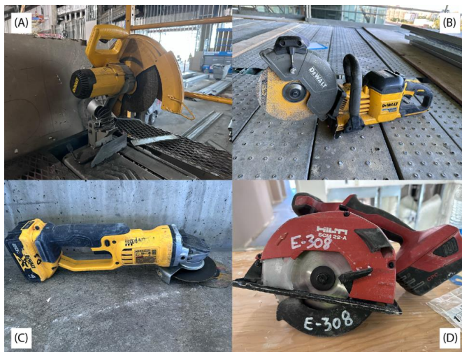
Fig. 3.1. Examples of each saw type that was used at the study sites. A = Chopsaw; B = Cut-off Saw; C = Grinder; D = Cordless Circular Saw.
