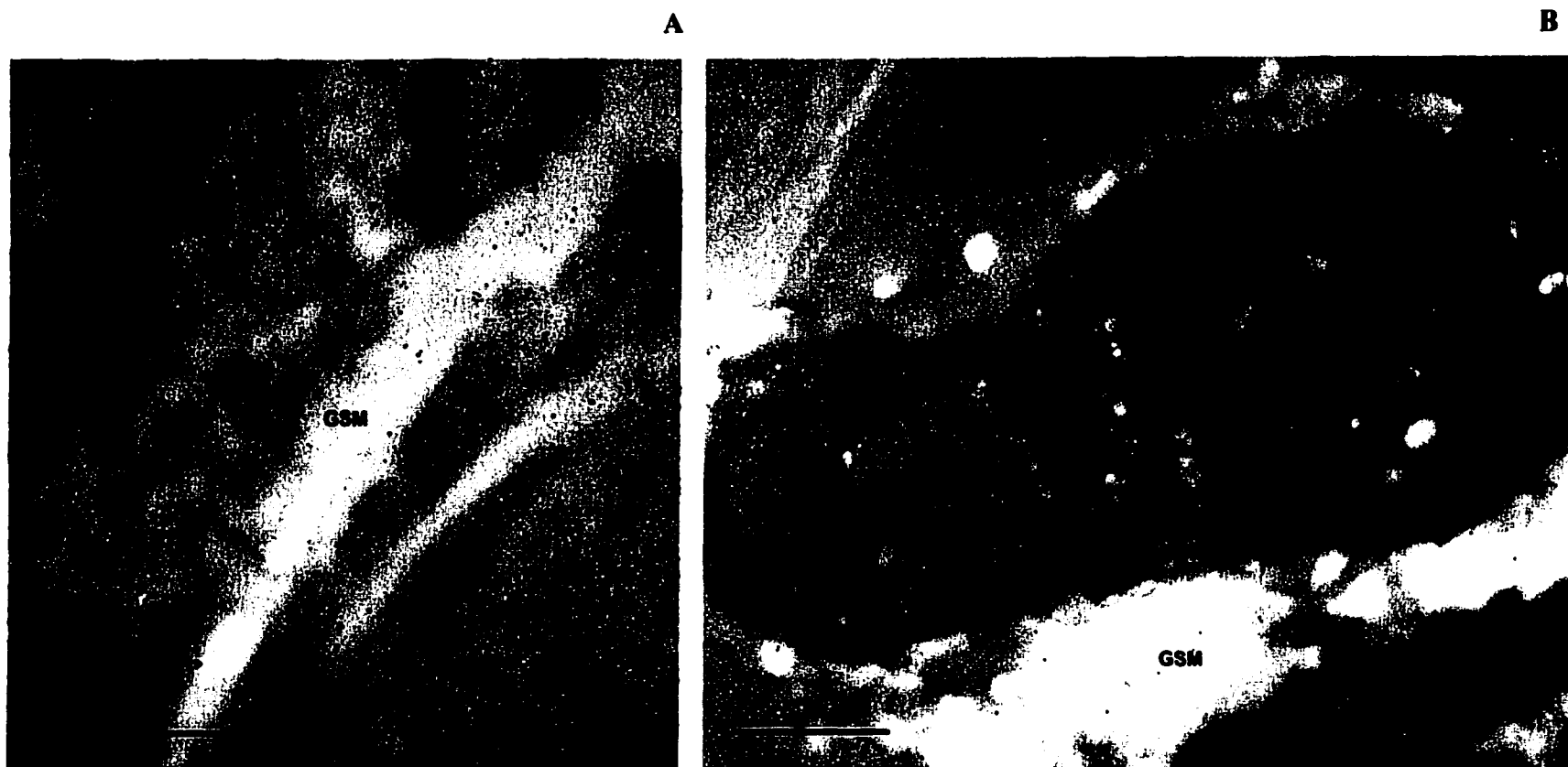
Figure 3.11. Transmission electron micrographs of normal (A) and QPM (B) corn grits extruded at specific mechanical energy of approximately 320kJ/kg. Protein aggregates (PA) appeared as large masses containing both \alpha -zein and \gamma -zeins, which were immunolabeled with colloidal gold particles of 12nm and 18nm diameter, respectively. The gelatinized starch matrix (GSM) can also be observed in the images. Bar = 1 \mu m
