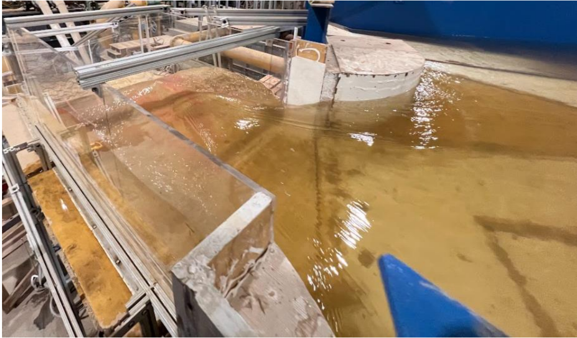
Figure 3-11. An illustration of flow entering the spillway for the spillway entrance fitted with circular abutments.
