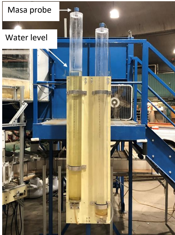
Figure 3-5. The Masa probe placed on the water-standpipes to monitor water-surface elevation in the headtank for the reservoir adjoining the spillway.
