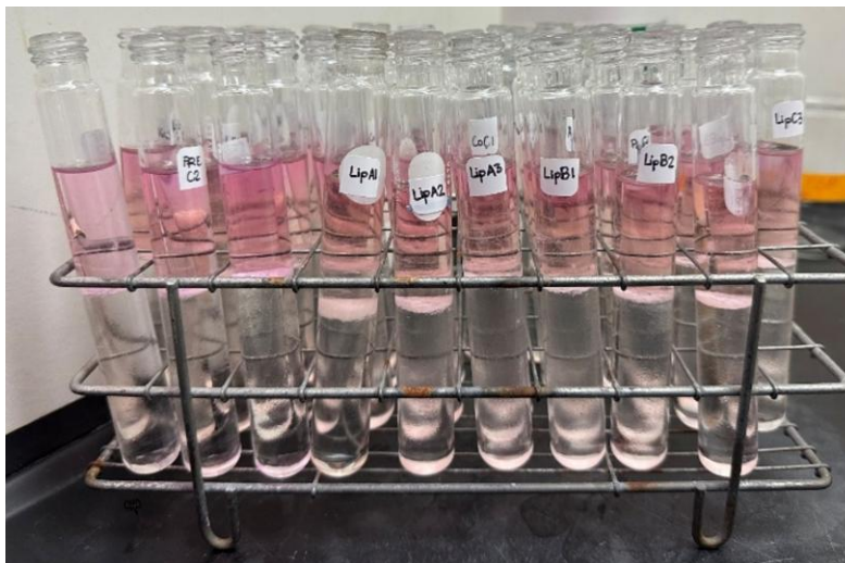
Figure 2-7. Picture of samples after Day 1 of Folch crude fat analysis demonstrating phase separation.
