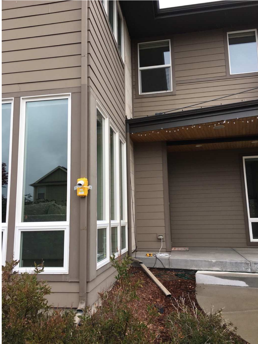
Figure 1. UPAS with weather resistant enclosure mounted to participant home.
