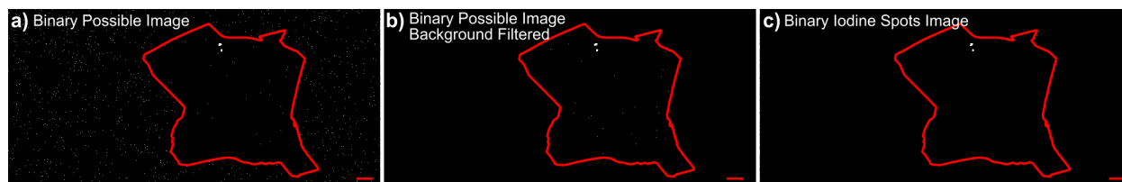
Figure S3.13: Iodine deposition spot identification and filtering. (a) A binary image of the nanoflake where all possible iodine deposition pixels are marked in white (pixel values of 1). (b) The same image as (a) after the first round of filtering that removes any possible spots in the background. (c) The final binary iodine spots image after the last filtering step, see SI text for details. The red line indicates the boundary of the nanoflake in all panels.
