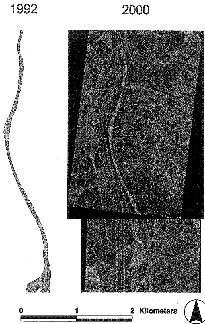
Figure 6.8: Digitized non-vegetated channel in 1992 (left) and 2000 aerial photo (right) of the upstream, narrow reach. This reach is located between A and B in Figure 6.5.
