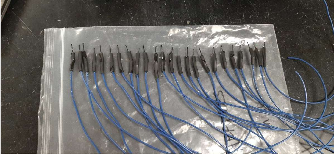
Figure 10. Epoxy curing overnight.
