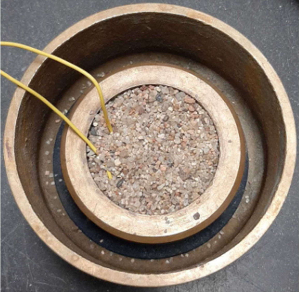
Figure 27. Sensors in the test cell covered with sand before compression.
