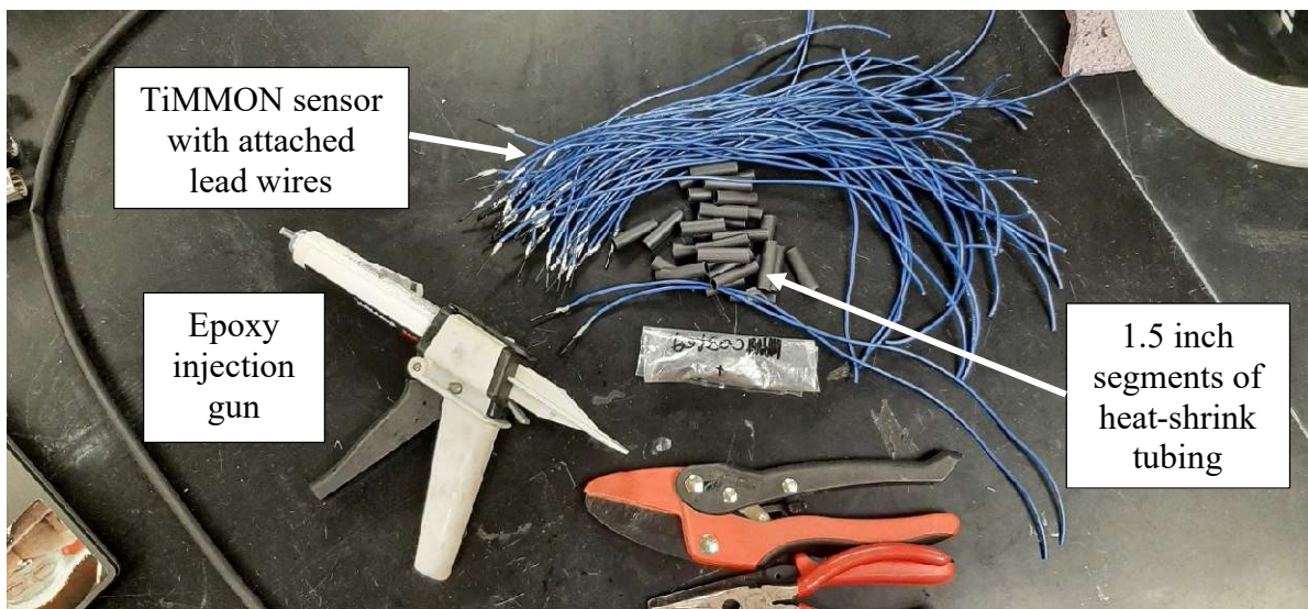
Figure 9. Sensors with electrical connections ready to be insulated and relevant tools.
