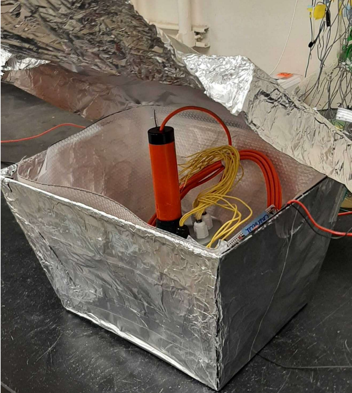
Figure 23. Apparatus and pH Meter V1.1 inside of Faraday cage.
