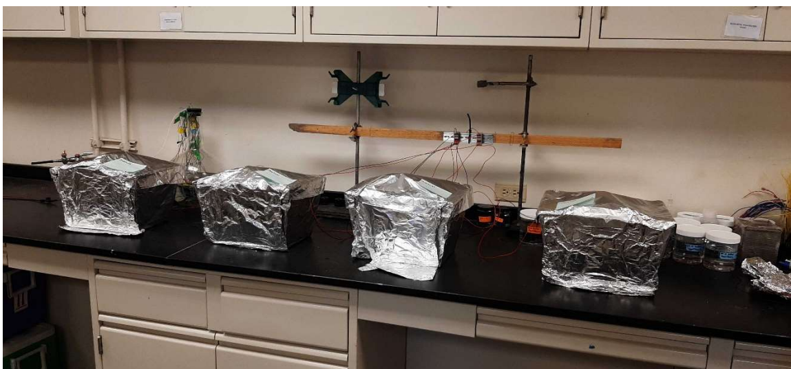
Figure 22. Faraday cages used with pH Meter V1.1.
