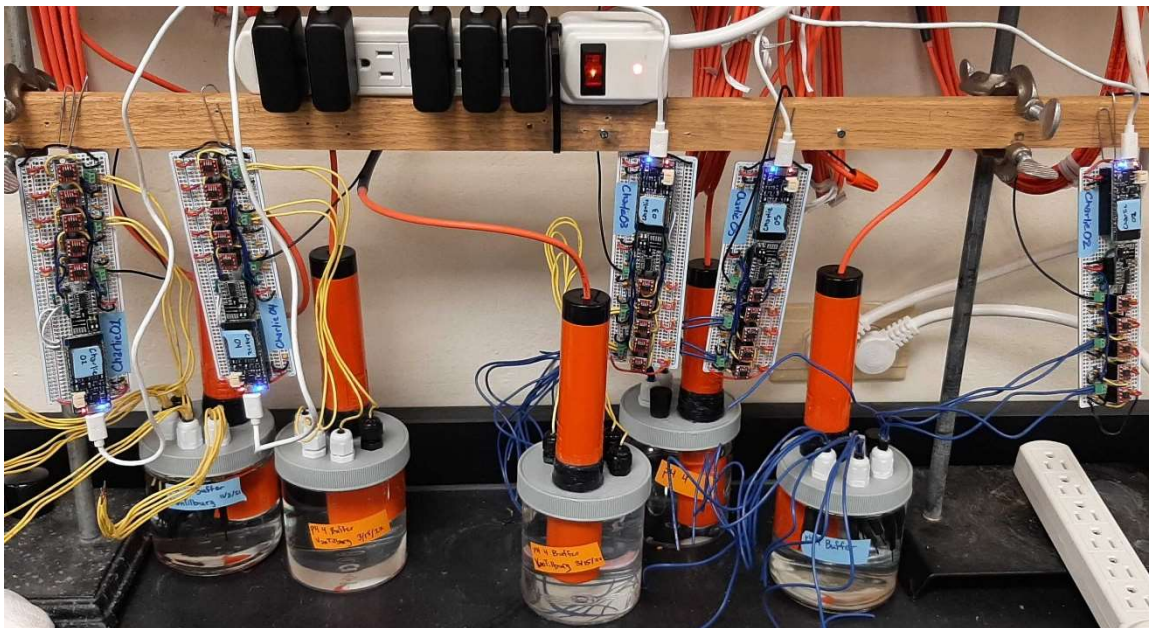
Figure 21. Five jar apparatuses used in the stepwise pH change experiments with sensors seen attached to the pH Meters V1.1s.
