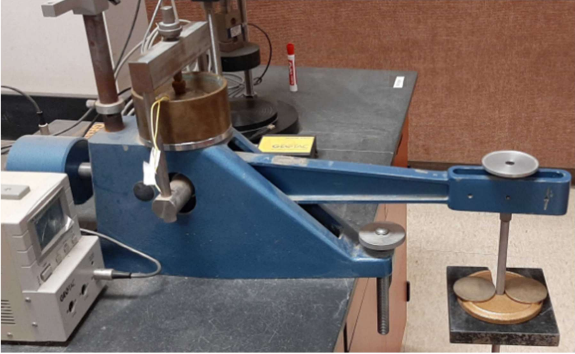
Figure 29. Soil oedometer frame with test cell inside and weights applied to the moment arm.
