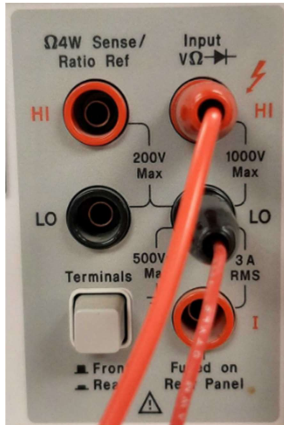
Figure 25. HP34401A Multimeter leads connected to the correct ports for measurement.
