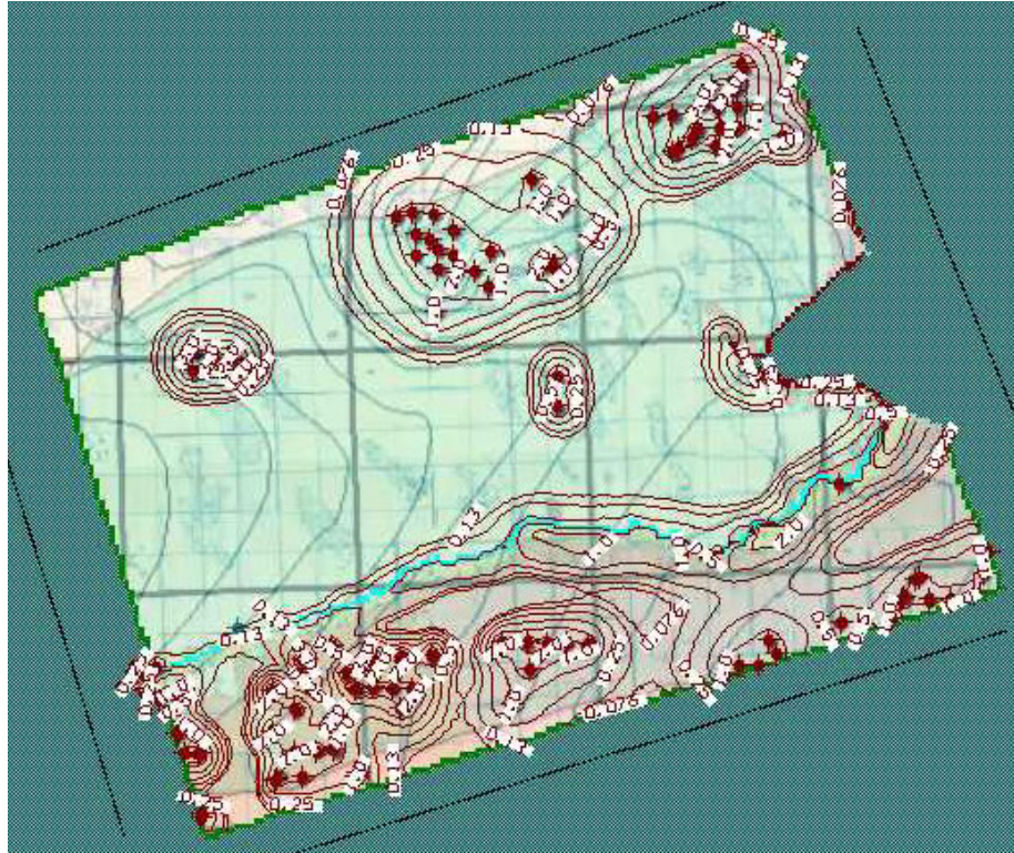
Figure 5-4: Cumulative Seasonal Drawdown, Irrigation and ET at the end of the growing season (day 257) (Visual Modflow v. 4.0 2003)
