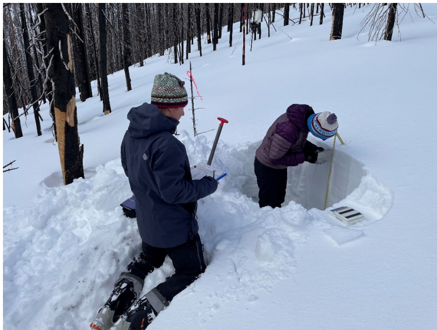
Figure 2: Manually measuring snow density, depth, temperature, permittivity, grain size, hardness, wetness, and SWE for individual snow layers within a snowpit during the 2024 melt season.
