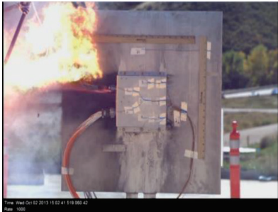
Figure 46. COTS-based secondary lithium-ion battery purposely subjected to cell overcharge to observe its reaction and to provide data to validate a thermal model [46].
