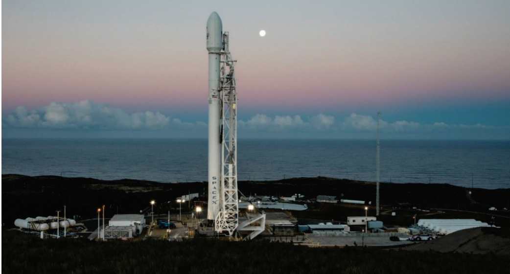
Figure 18. SpaceX Falcon 9 launch vehicle in a vertical position at the Vandenberg Space Force Base being readied to launch the Iridium-1 satellite into orbit [58].
