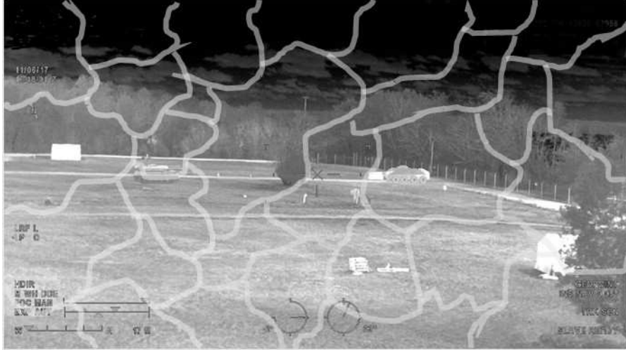
Figure 3-9: Concept Illustration of Random Distribution of Isoplanatic Patches Across the Field of View.
