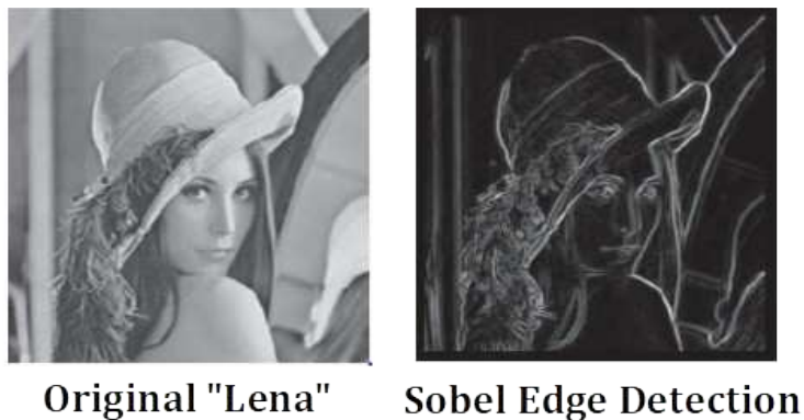
Figure 3-15: Example of Sobel Edge Detection Processing
