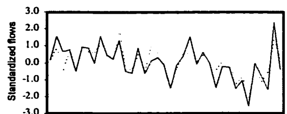
Fig. 6-9c Performance MLR-LAD of 3 predictors for Nile River flows at Aswanduring the Calibration (1953-1972), validation (1973-1989)
