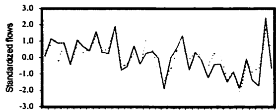
Fig. 6-9a Performance MLR-LAD of 3 predictors for the Blue Nile River flows during the Calibration (1953-1972), validation (1973-1989)
