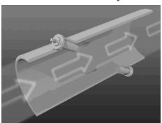
and downstream. The time it takes for the sound to travel from one transmitter to the other is precisely measured. Velocity measurement is accomplished by comparing the time the sound wave takes to travel with the flow versus against the flow ( $\Delta$  Time). Some transit time flowmeters (generally permanent installations) make use of multiple acoustic paths to better sample the flow profile.
