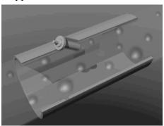
relation to the pipe. The transducer generates and focuses an ultrasonic sound wave into the fluid. Suspended particles or air bubbles within the media reflect the sound waves back to the transducer, which now acts as a receiver listening for the return echo. The delay in the echo is measured and directly correlates to the velocity of the particle, which is assumed to be equal to the fluid velocity.
