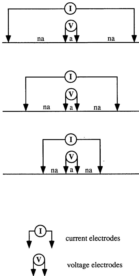
A Schlumberger array consists of two voltage electrodes placed a distance 'a' apart, and two current electrodes, one on either side of, and a distance 'na' (some multiple 'n' of 'a') from of the voltage electrodes. A Schlumberger depth sounding entails changing the position of the current electrodes (changing 'n'); the farther they are apart, the deeper the measurement, the closer they are together, the shallower the measurement.
