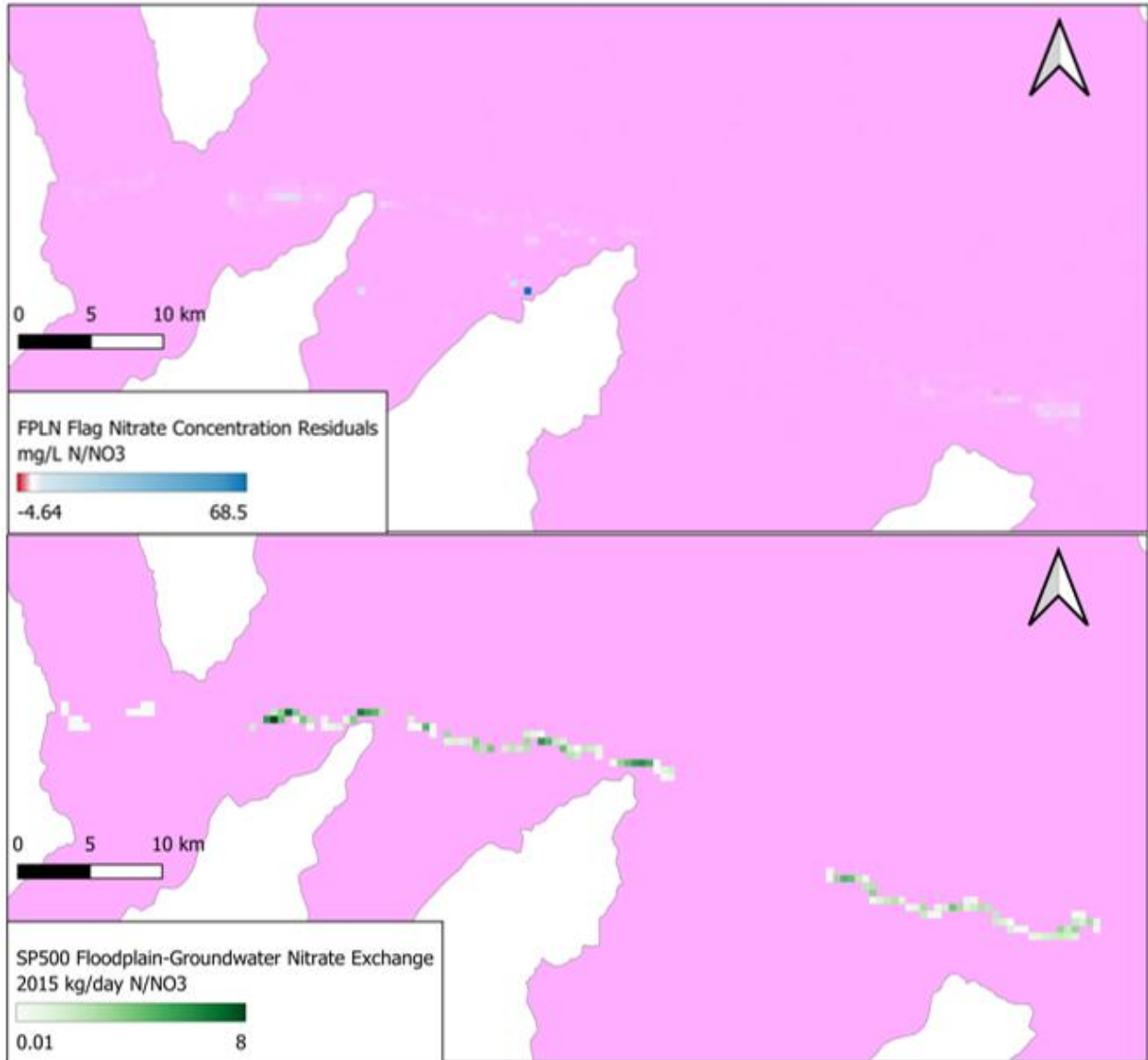
Figure C.2: Top map shows groundwater nitrate concentration residuals during the SP500 scenario from modeling with and without the floodplain flag. Bottom map includes simulated masses of nitrate loading through floodplains during 2015 of the SP500 scenario.
