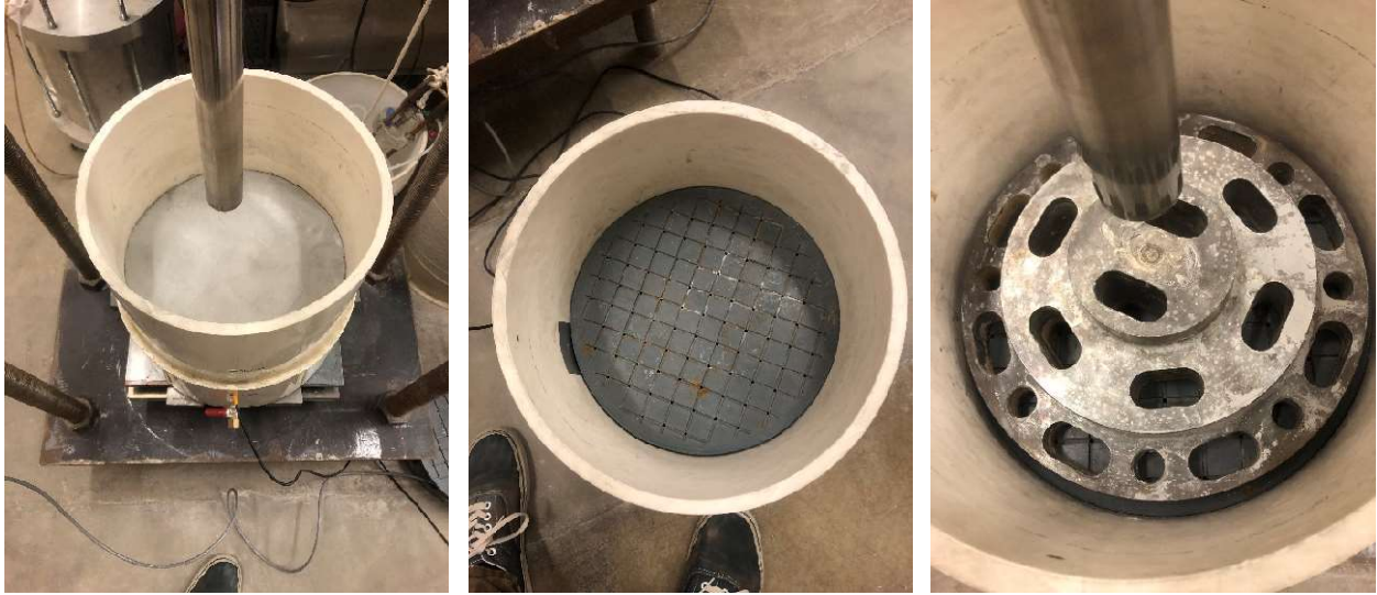
Figure 9. Specimen constructed in large mold being prepared for compression testing.
