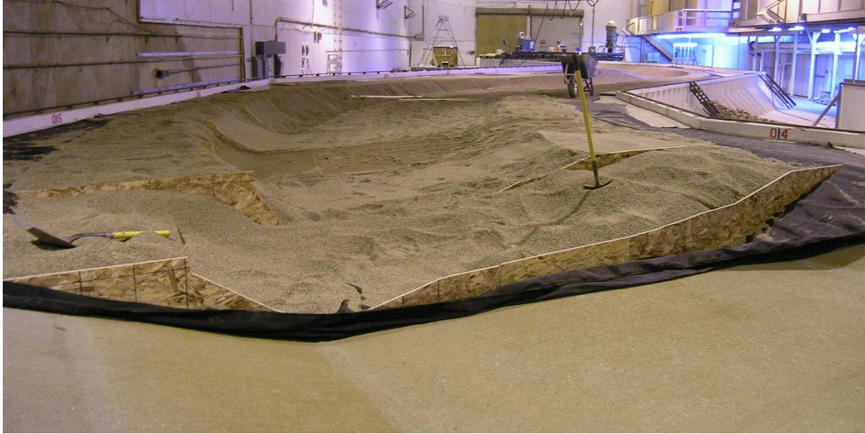
Figure 7. Construction of the native topography channel
