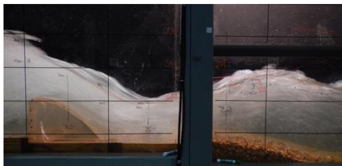
b) 1:36 Scale Section Model
