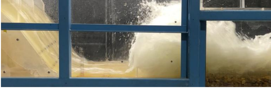
Figure 137. Jump Action Lost, Lower Unit Discharge (High Froude)
