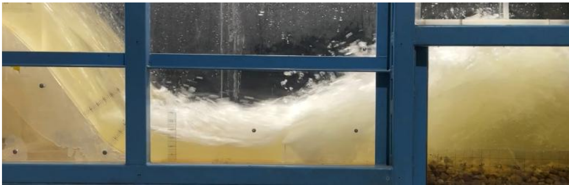
Figure 137. Jump Action Lost, Lower Unit Discharge (High Froude)
