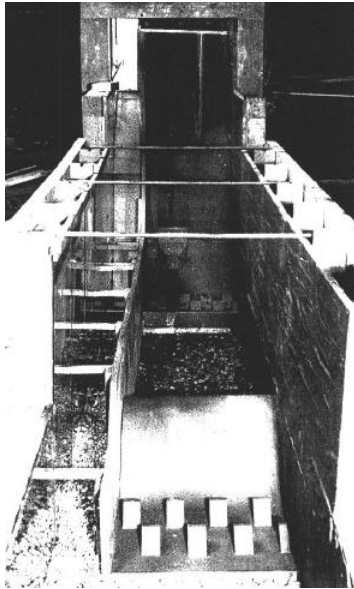
b) 1:36 scale model (iso view)
