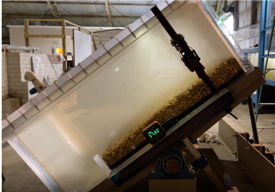
Figure 77. Tilt-Flume for use in determining submerged angle of repose of bed material (Coarse Gravel Material)
