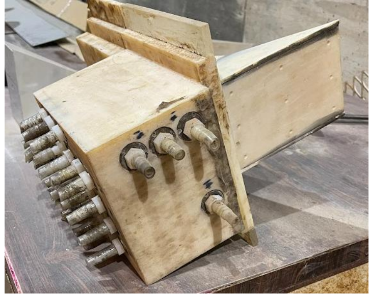
b) Pressure Tap Configuration
