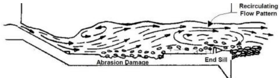
a) Problematic Flow Pattern Entraining Materials
