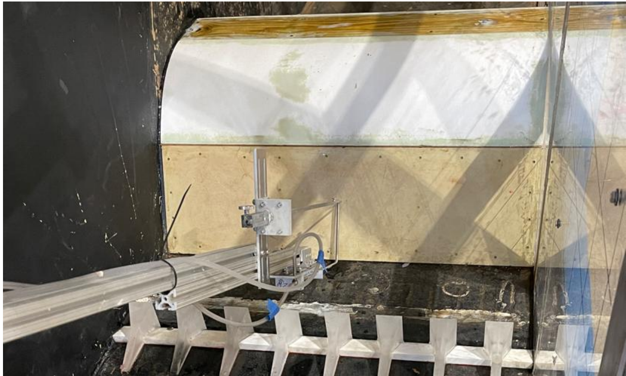
Figure 157. Incoming Flow Instrumentation with Low Crest
