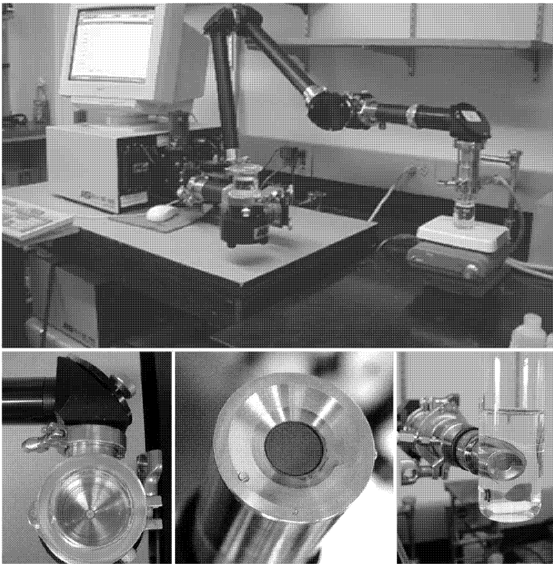
Figure 1.1. Instrument and ATR Probes used for ATR-FTIR Spectroscopy. Top. ReactIR-1000, ATR-FTIR spectrometer from Mettler-Toledo, connected to a computer and the ATR probes. Bottom, left. Top view of the Diamond probe, showing the Di crystal in the center of the stainless steel enclosure. Bottom, center. Silicon probe detail showing a \text{DEC}^+\text{NO}_3^- film on the Si crystal and 1 mL of water used for equilibration. Bottom, right. Silicon probe, shown on the side, with a custom glass container attached.
