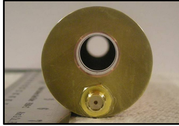
Figure 2.20: Schematic and pictures of the endcap for the rf region, all dimensions are in inches. On the left is the side view of the endcap and on the right is the view looking down the beam path.
